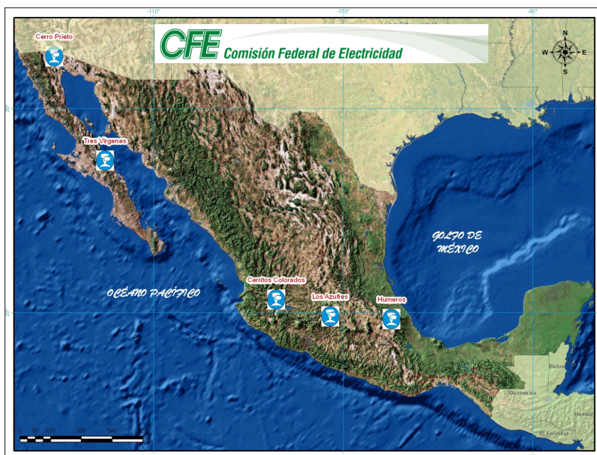
FIGURE 3: Locations of Mexican geothermal fields under exploitation (Cerritos Colorados, formerly known as La Primavera, remains in stand-by). The national capacity factor in 2013 was 80.6% or 0.8 on average. All the fields and power units are managed and operated by personnel of the CFE.
