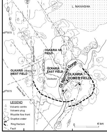
FIGURE 3: Structural map of Olkaria geothermal field
