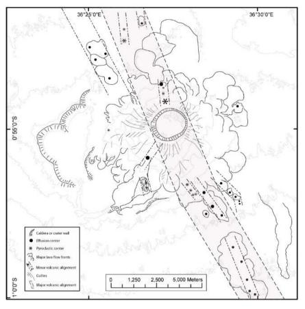
FIGURE 8: Structural map of Longonot prospect
