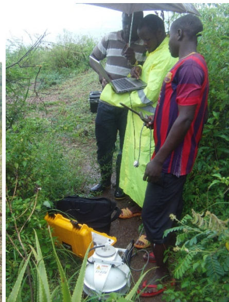
FIGURE 11: Soil gas sampling
