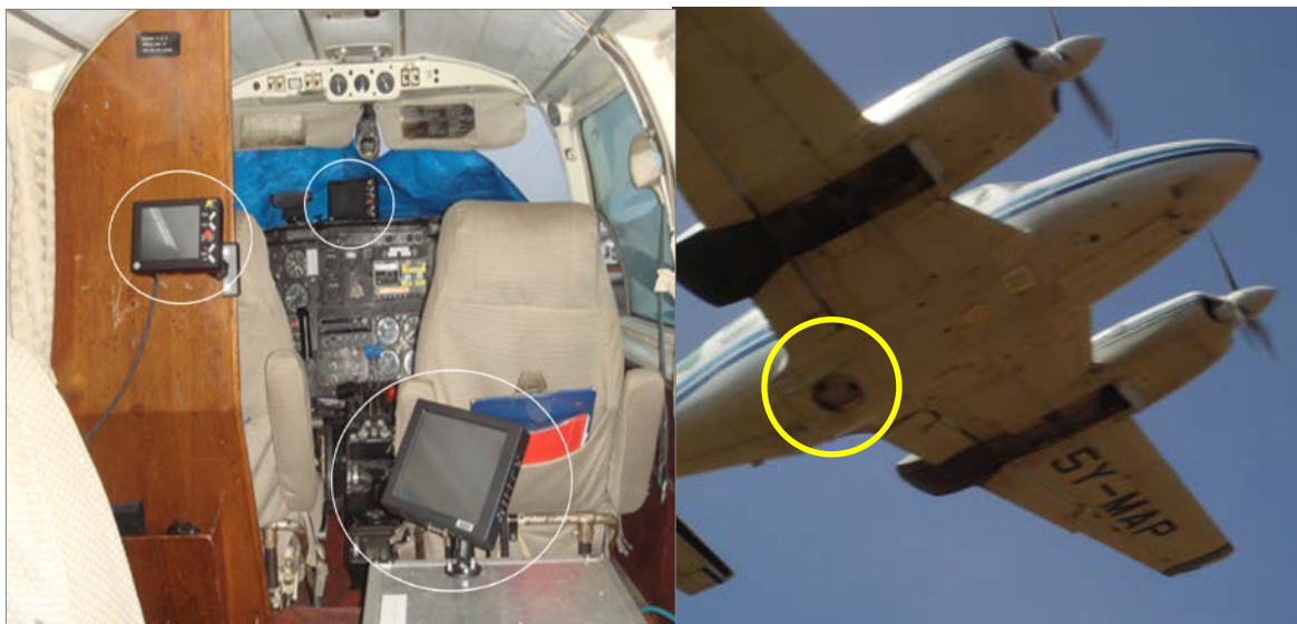
FIGURE 3: Touch screen monitors for operating the Thermal camera and the camera hatch as seen from below the aeroplane
