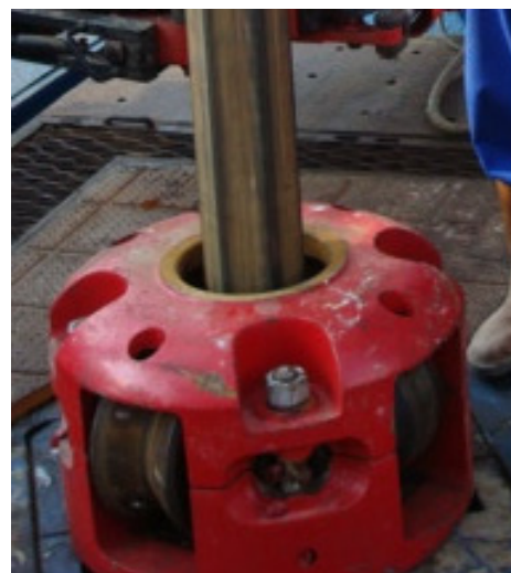
FIGURE 16: Kelly fitted into a drive bushing
