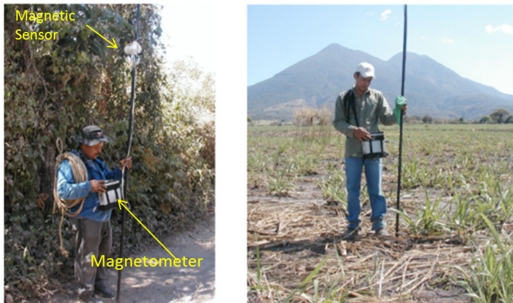
FIGURE 11: Examples of a field measurement with a magnetometer model GEM-19T from GEM System, owned by LaGeo; a magnetic survey in the San Vicente volcano area
