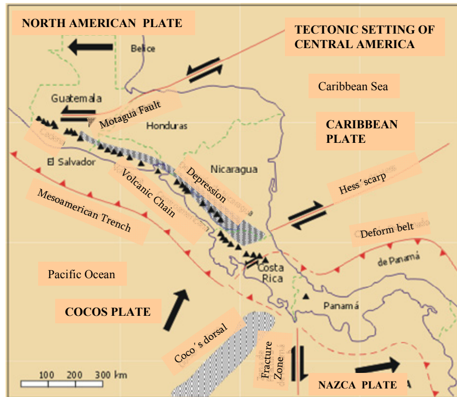
FIGURE 1: Subduction of the Cocos plate over the Caribbean plate and the volcanic chain (Source: modified from CEPREDENAC)
