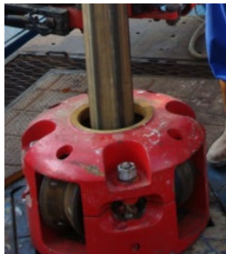
FIGURE 16: Kelly fitted into a drive bushing
