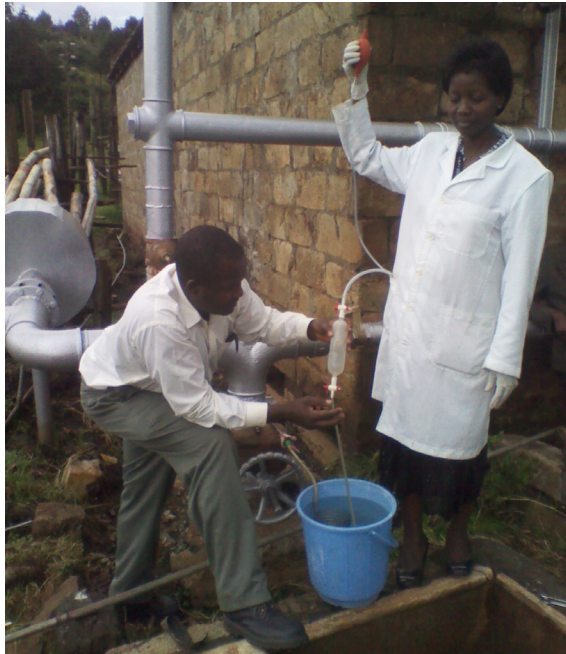
FIGURE 15: Gas and condensate sampling
