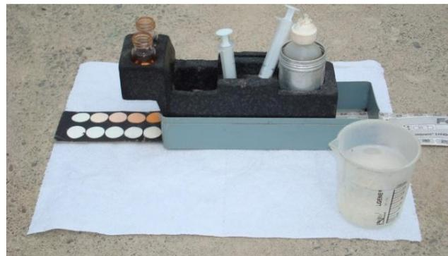
FIGURE 12: Colorimetric traditional method. Photo by P. Moya
