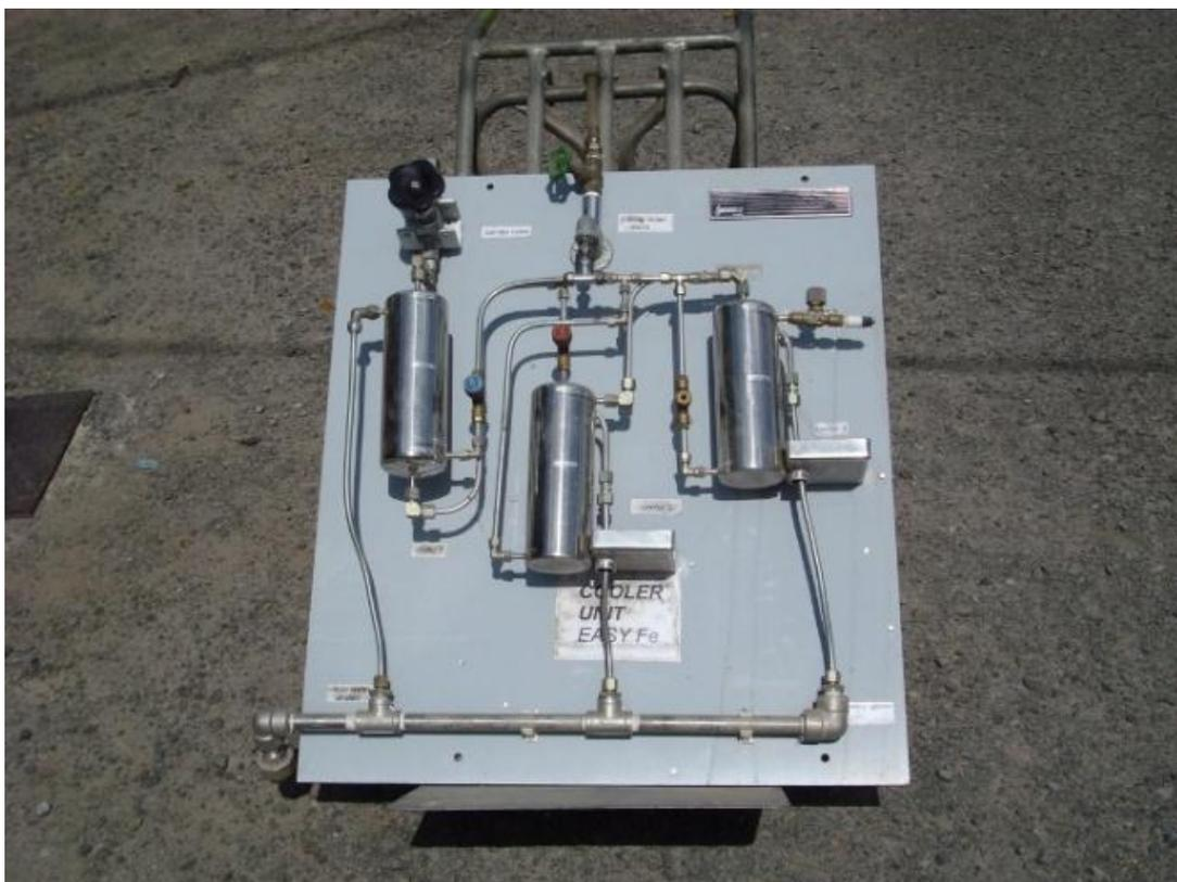
FIGURE 6: System to process the brine sample. Photo by P. Moya
