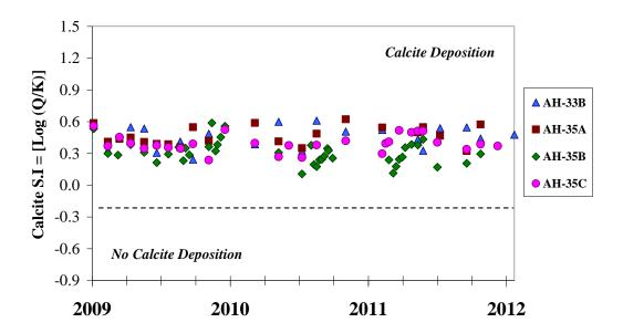
FIGURE 1: Calcite saturation index of wells AH-33B, AH-35A, AH-35B and AH-35C
