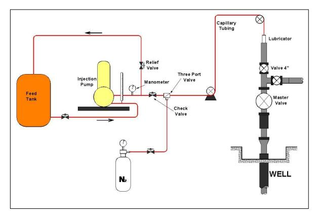
FIGURE 2: The calcite chemical inhibition system
