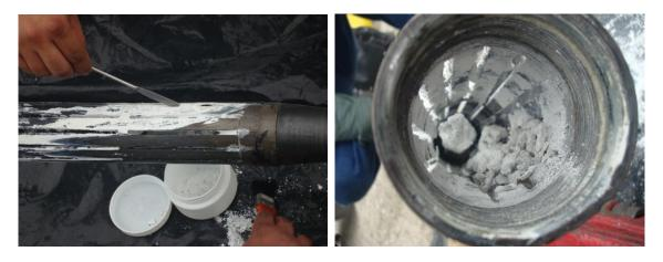
FIGURE 4: Inhibitor's solid by-products deposited in the injection system.
