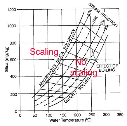
FIGURE 2: Solubility of silica in water. Scaling occurs above the amorphous silica solubility curve.
