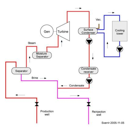
FIGURE 3: Sketch of the fluid path of a conventional geothermal power plant with a surface condenser
