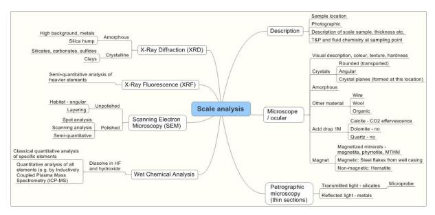
FIGURE 1: Methods used for geothermal scale analysis
