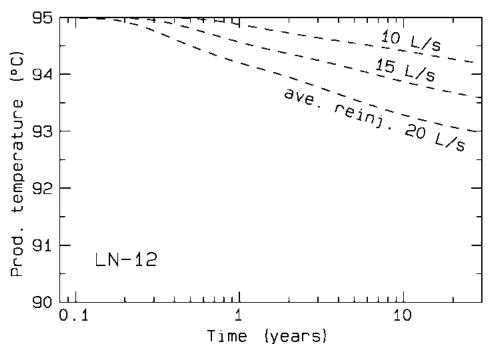
FIGURE 13: Estimated production temperature decline of well LN-12, due to flow through the three channels simulated (Figure 12), for three cases of average long-term reinjection into well LJ-8 and an average long-term production rate of 40 L/s (figure from Axelsson et al., 2001)
