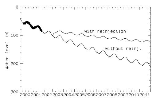
FIGURE 3: Water level predictions for the Hofsstadir low-temperature system in W-Iceland (Axelsson et al., 2005b). Both predictions assume the same production, while one assumes full reinjection and the other no reinjection. See Hofsstadir discussion later in the paper
