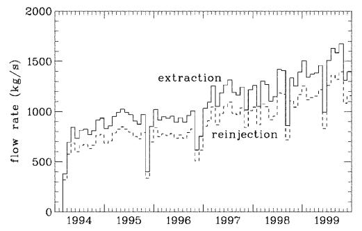
FIGURE 6: Extraction- and reinjection history of the Miravalles high-temperature field in Costa Rica 1994 – 1999. Since then production and reinjection has increase as installed capacity has increased from 125 MW<sub>e</sub> in 1999 to 163 MW<sub>e</sub> (see also Moya and Nietzen, 2010)
