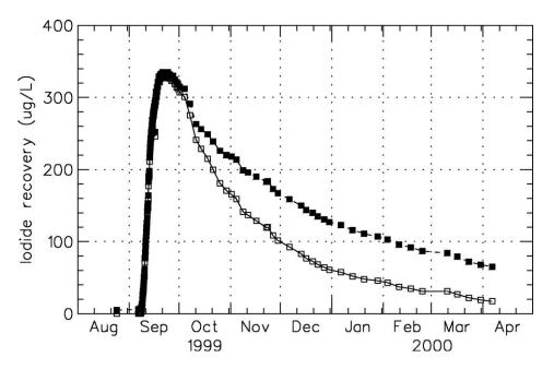
FIGURE 10: Iodide recovery in production well K-21 in the Krafla high-temperature system in N-Iceland, following the injection of 200 kg of KI into well K-22 (from Axelsson, 2011. The test lasted 7 months. The lower curve shows the recovery corrected for the tracer being reinjected (recirculated) after production. About 30% of the tracer was recovered during the test)
