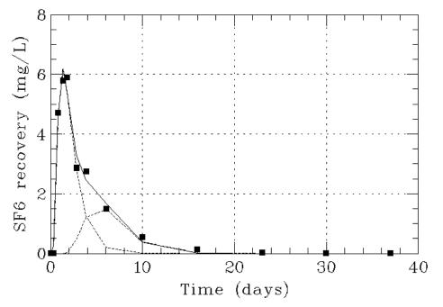
FIGURE 14: Observed and simulated (two flow channels) SF<sub>6</sub> recovery in well AZ-5 in the Los Azufres high-temperature field in Mexico, following injection into well AZ-64 200 m away (Molina-Martínez and Axelsson, 2011). The very rapid recovery is attributed to steam-phase transport. Almost 50% of the tracer was recovered through a combined flow channel volume of 200,000 m<sup>3</sup> (~10% porosity)
