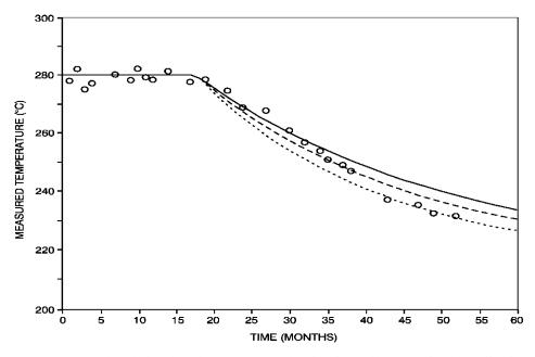
FIGURE 8: Measured and simulated temperature decline in well PN-26 in the Palinpinon field, Philippines (from Malate and O'Sullivan, 1991)
