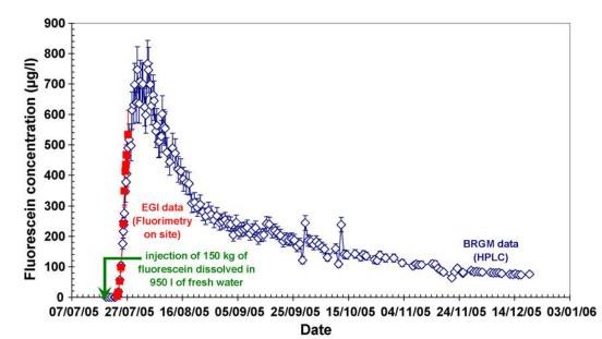
FIGURE 11: Flourescein recovery in well GPK-2 at the Soultz EGS-site in N-France, following the injection of 150 kg of fluorescein into well GPK-3 (figure from Sanjuan et al., 2006). The test lasted 5 months. About 24% of the tracer was recovered during the test
