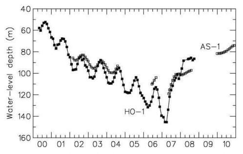
FIGURE 7: Pressure changes in the Hofsstadir low-temperature geothermal system in W-Iceland during the first 11 years of production, shown as water-level changes in the main production well (HO-1) and in a monitoring well (AS-1). A continuous pressure decline for 7 years is reversed in the spring of 2007 when reinjection commences. Figure from Axelsson (2011)
