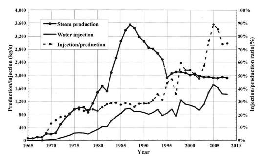
FIGURE 4: Steam production and water injection history of the Geysers geothermal field in California (Goyal and Conant, 2010)
