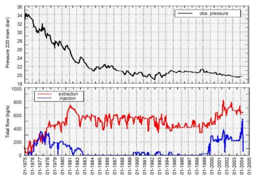
FIGURE 5: The production, reinjection and pressure response history of the Ahuachapan geothermal system in El Salvador (see also Monterrosa and Montalvo, 2010)
