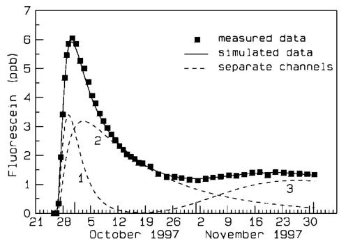
FIGURE 12: Observed and simulated (three flow channels) fluorescein recovery in well LN-12 at Laugaland in N-Iceland during a tracer test in 1997 (figure from Axelsson et al., 2001). Spent geothermal fluid was reinjection into well LJ-08 and production was from well LN-12 about 300 m away. According to the simulation only about 6% of the tracer injected is recovered through this well and the combined flow-channel volume is estimated as 20,000 m<sup>3</sup>, assuming 7% porosity
