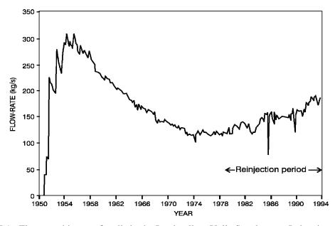
FIGURE 1: Flow-rate history of wells in the Larderello – Valle Secolo area, Italy, since the early 1950's demonstrating the benefit of reinjection (from Capetti et al., 1995)
