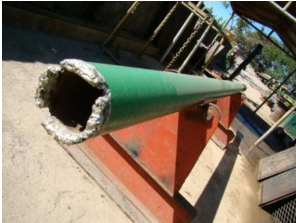
FIGURE 11: Crown mill of 5" x 3 1/2"
