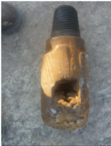
FIGURE 1: Side view of 5 7/8" bit-mill
