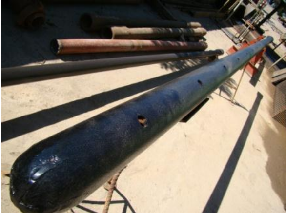
FIGURE 9: Tube diffuser of 3 ½"
