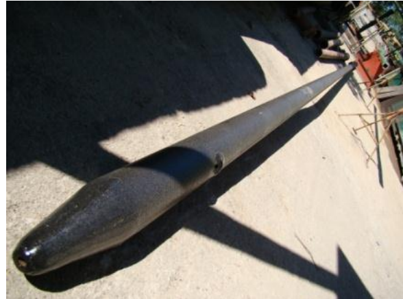
FIGURE 10: Pipe jet of 3 ½"
