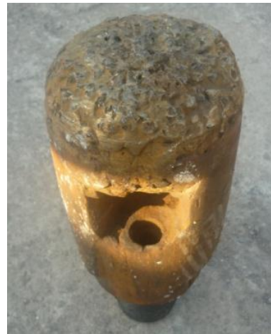
FIGURE 2: Top view of 5 7/8" bit-mill
