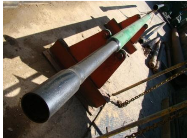
FIGURE 12: Joint of Crown mill of 5" x 3 1/2"
