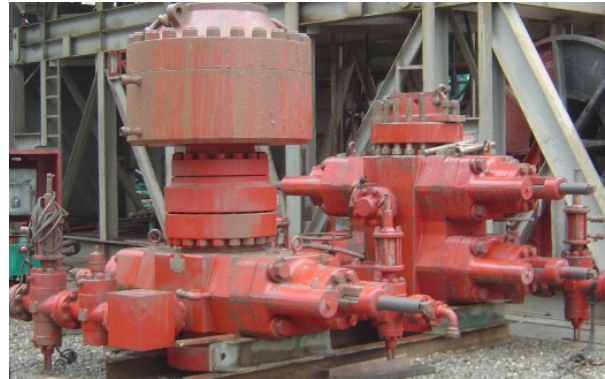
FIGURE 22: Two BOP stack
