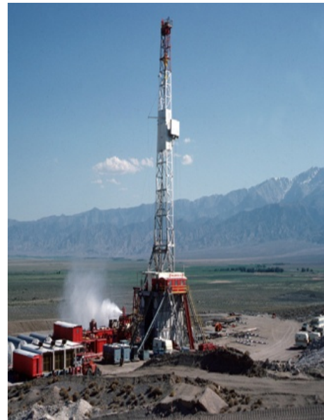
FIGURE 20: Typical conventional rig
