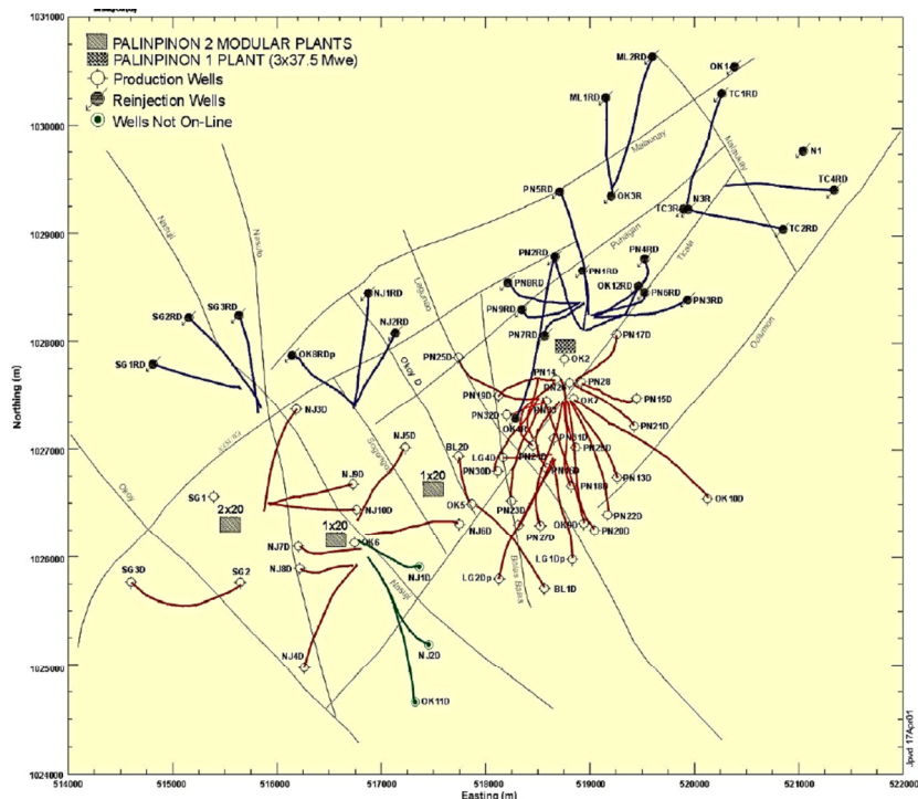
FIGURE 10: Map of the Palinpinon geothermal field in the Philippines showing directional well tracks and locations
