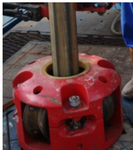
FIGURE 16: Kelly fitted into a drive bushing
