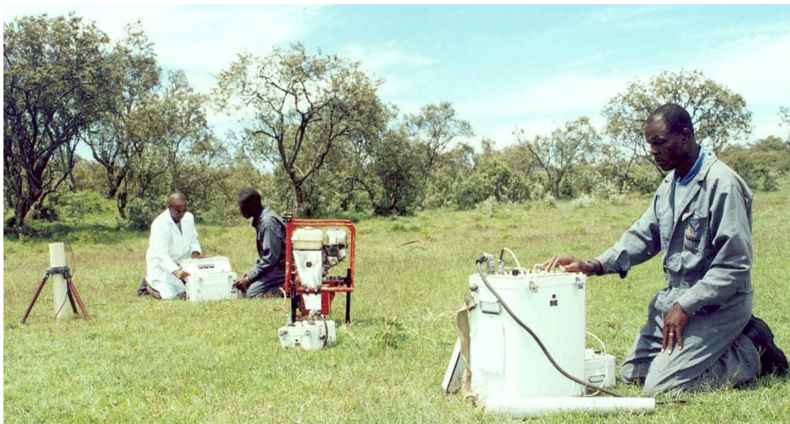
FIGURE 1: TEM System in Operation
