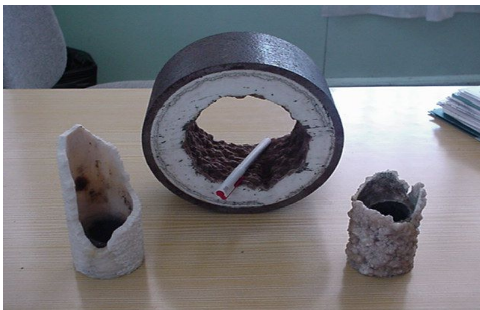
FIGURE 3: Calcium carbonate encrustations, PGM-01 Miravalles
