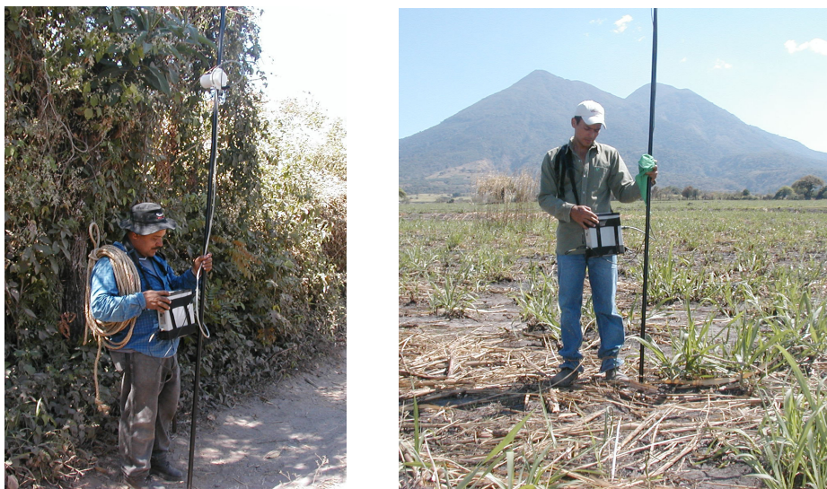
FIGURE 7: Examples of a field measurement with a magnetometer model GEM-19T from GEM System, owned by LaGeo; a magnetic survey in the San Vicente volcano area
