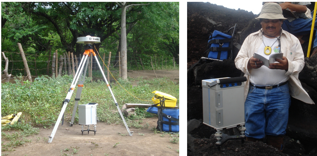
FIGURE 1: A) Gravity at a base station opening loop, together with a remote reference GPS; B) A site measurement, gravity and position using double frequency GPS are measured
