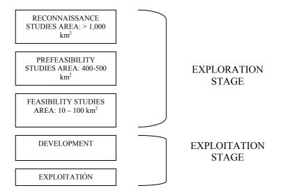
FIGURE 1: Exploration and exploitation stages in a geothermal project
