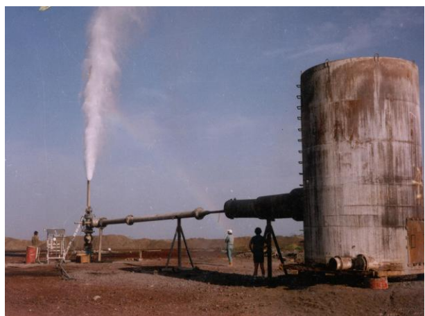
FIGURE 3: Shallow well (TD-5) in the Tendaho geothermal field. Total depth = 516m; max. temp. = 253°C
