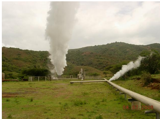
FIGURE 2: Discharging well (LA-3) in the Aluto-Langano geothermal field. Total depth = 2.3Km; max. temp. = 320°C
