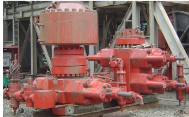
FIGURE 22: Two BOP stack
