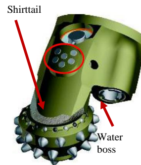
FIGURE 7: Bit body (single leg) with cone and bearing in place
