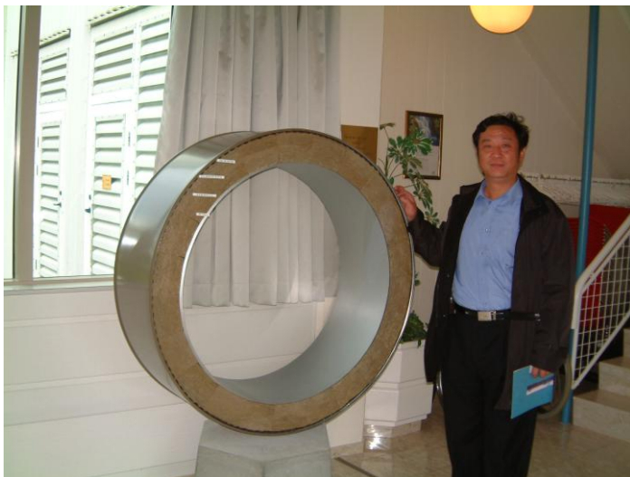
FIGURE 12: Pipeline made of steel, insulated with rock wool covered with plastic and aluminium on the outside where the pipeline lies above ground, but with urethane insulation, covered with plastic, where it runs underground.
