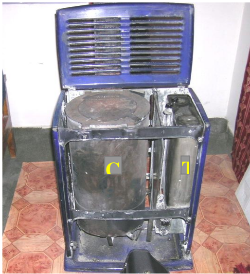
FIGURE 4: A typical 'Bukhari' traditionally used in Leh for space heating during winter. Kerosene from a storage tank (T) is pumped into a closed hollow cylinder (C). Kerosene burns continuously in the cylinder radiating heat into the space outside. The exhaust (mostly CO 2 ) is released into the atmosphere through an exhaust tube connected to the cylinder.
