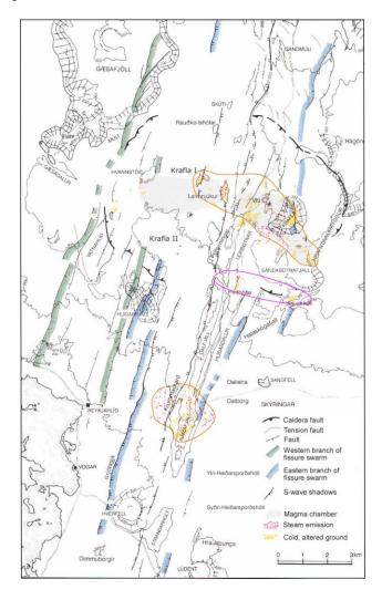
FIGURE 5: Central part of Krafla volcanic system showing caldera and fissure swarms which traverse it. The Krafla caldera hosts a geothermal system. It has a magma chamber (s-wave shadow) at 3-7 km depth. A second geothermal area at Námafjall on the fissure swarm 7 km south of Krafla is located where basaltic fissure eruptions concentrate.
