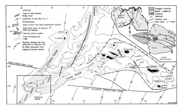
FIGURE 7: High-temperature geothermal fields on the Azores Islands are related to flank zone volcanism north of the Azores Fracture Zones. They developed in caldera regions of stratovolcanoes. Prominent fissure swarms formed in the direction of max. stress
