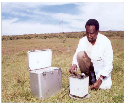
FIGURE 14: Gravity measurements using a La Coste gravimeter at Olkaria Geothermal field.
