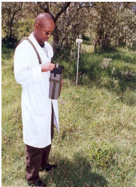
FIGURE 12: Magnetic data collection using a magnetometer
