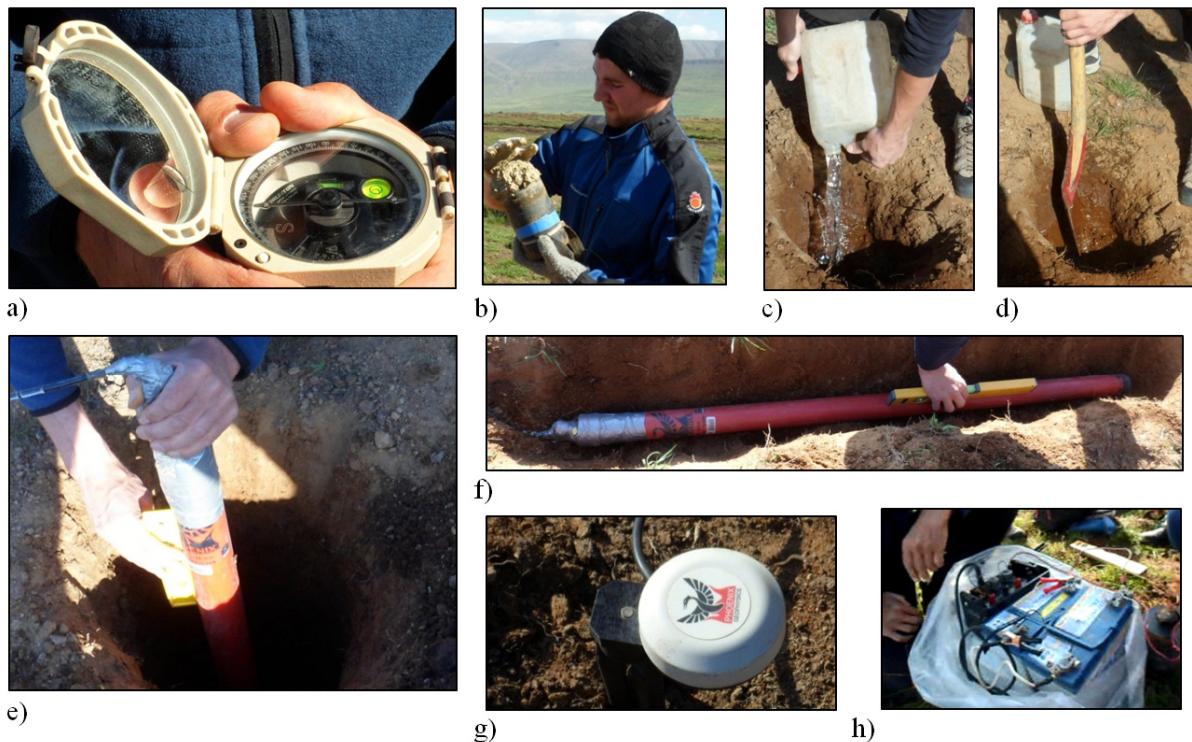
FIGURE 19: Field layout for MT measurements, a) Setup of true North direction; b) Adding bentonite to the electrode; c) Adding saltwater into the hole; d) Making a hole; e) Placing the vertical induction coil; f) Placing the horizontal induction coil; g) Placement of GPS; h) Instrument connection with the battery
