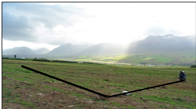
Field set up of Large Receiver coil (10 x10 m, effective area of 5613 m 2 )
