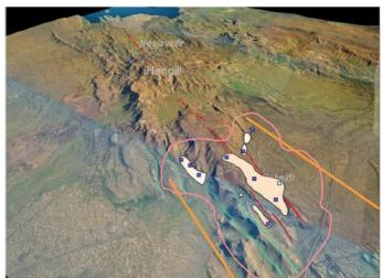
FIGURE 14: Map of the Hengill area showing Hellisheidi geothermal field; volcanic fissures are red, green lines indicate main faults; between yellow lines are several production fields; pink area shows where drill holes can be located with minimum impact on the environment; blue squares show the location of well platforms (Gunnlaugsson et al., 2010)
