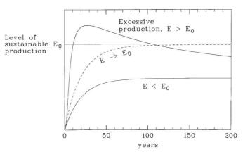
FIGURE 5: Sustainable production from a geothermal system (Axelsson et al., 2001)
