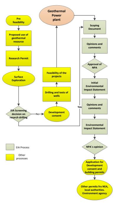
FIGURE 9: Simple geothermal developmental regulatory framework (modified from Gunnlaugsson, 2008)
