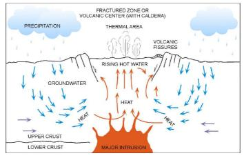
FIGURE 4: A general conceptual model of a high temperature field (Steingrímsson, 2012)
