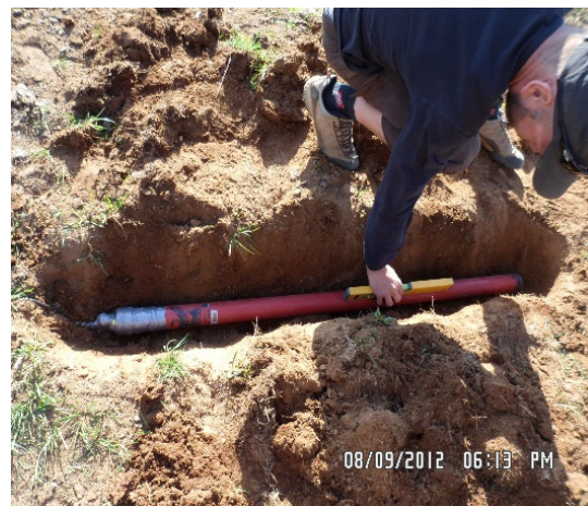
FIGURE 13: Levelling of the magnetic coil (field work with ISOR, 2012)
