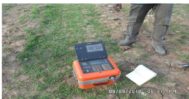
FIGURE 10: Digital receiver (used in field work in N-Iceland, 2012)
