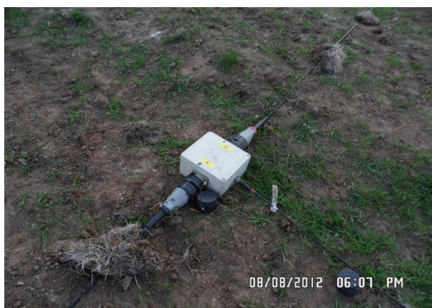
FIGURE 11: Connection of receiver loop to digital receiver (photo from field work in N-Iceland 2012)
