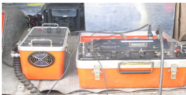
FIGURE 9: The power module connected to the transmitter (used in field work in N-Iceland, 2012)
