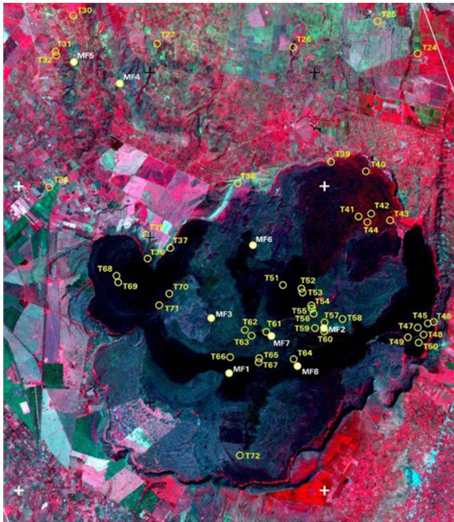
FIGURE 5: Hotspots in the Menengai geothermal field from infrared mapping (BGR, 2009)
