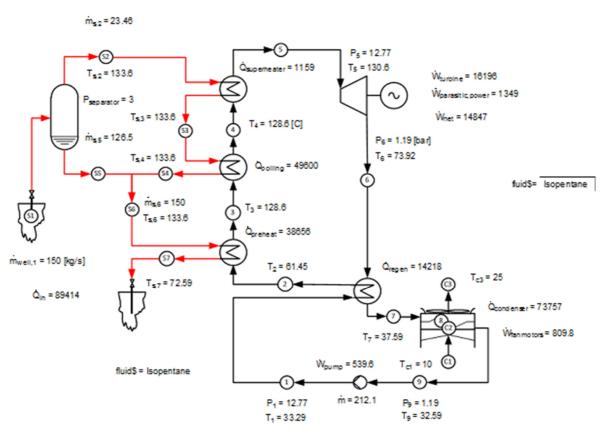
FIGURE 19: Schematic diagram of proposed binary plant with EES values, isopentane as working fluid
