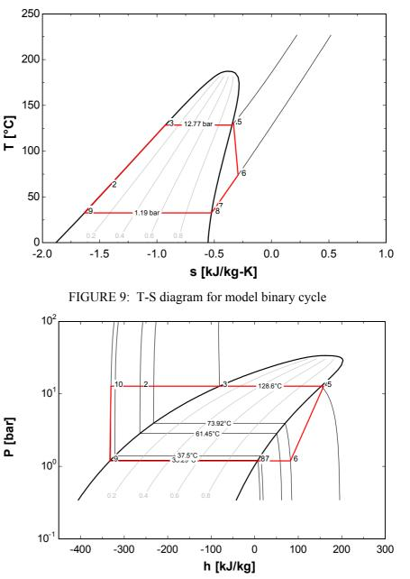
FIGURE 10: P-h diagram for model binary cycle
