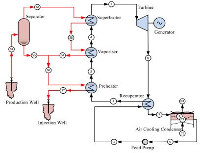
FIGURE 8: Schematic diagram of proposed binary plant with air cooling system
