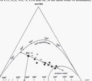
FIGURE 3: Na-K-Mg plot showing thermal discharges in various stages of partial equilibrium GW-2 discharge is the nearest representative of the Puga deep fluid, which has evidently Attained Na-K equilibrium at 255°C. The shallow reservoir temperature is indicated to be around 200°C (Ravi Shanker et al., 1999)
