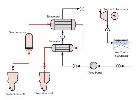
FIGURE 7: Schematic diagram of a basic binary cycle
