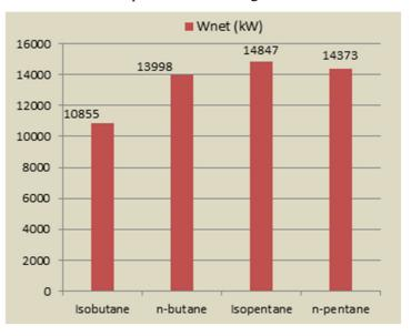
FIGURE 20: Net optimum output of the plant
