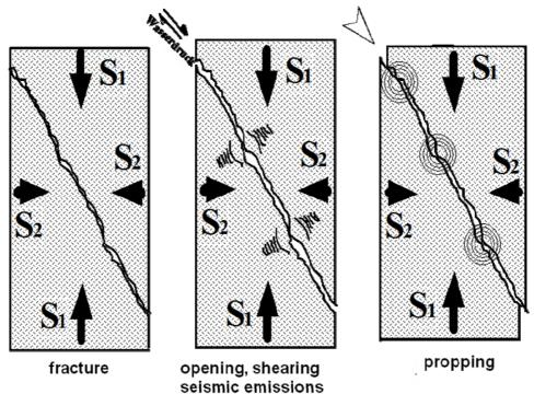
FIGURE 24: Selfpropping: Existing fracture at (1) initial state within a deviatory stress field with maximum stress magnitude S1 and minimum stress magnitude S2, (2) while injecting water and increasing the pressure, producing shearing, and seismic emissions, and (3) after pressure release and the self propping by new supporting points as illustrated (Jung 1999)
