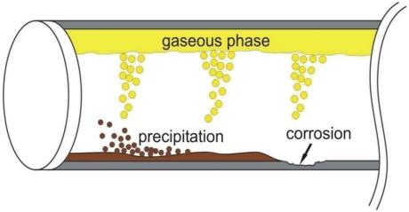
FIGURE 28: Probable processes during the circulation of thermal water
