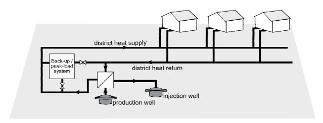
FIGURE 34: Scheme of a well doublet with backup/peak-load system feeding a district heating grid
