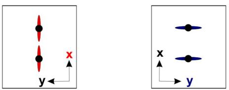
FIGURE 21: Conceptual arrangements of bottom hole positions in relation to fracture propagations. Left is a serial arrangement with fractures along the connection line of both wells and right, a parallel arrangement. Both wells in a thermal loop have in the serial arrangement dominantly artificial
