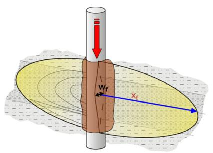
FIGURE 26: Artificial fracture generated by the hydraulic proppant frac technique with fracture width  $w_f$  and fracture length  $x_f$  in a normal faulting or strike-slip faulting tectonic regime (Figure 10)
