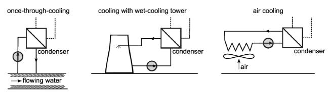
FIGURE 39: Chiller solutions for condensing purposes in the conversion plant (taken from Saadat et al., 2010)
