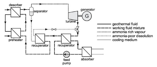
FIGURE 38: Schematic setup of a Kalina cycle (Saadat et al., 2010)
