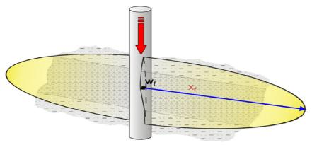
FIGURE 23: Artificial fracture with fracture width  $w_f$  and fracture length  $x_f$  generated by the waterfrac technique in a normal faulting or strike-slip faulting tectonic regime (Figure 10)
