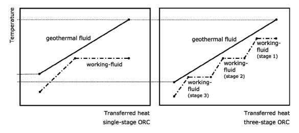
FIGURE 36: Example of a temperature-heat transfer-diagram for a single-stage and a three-stage ORC
