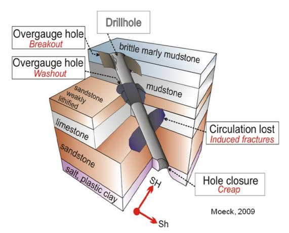
FIGURE 15: Potential geology related drilling problems (Moeck in Sperber et al., 2010). SH and Sh represents the direction of maximum and minimum horizontal stress
