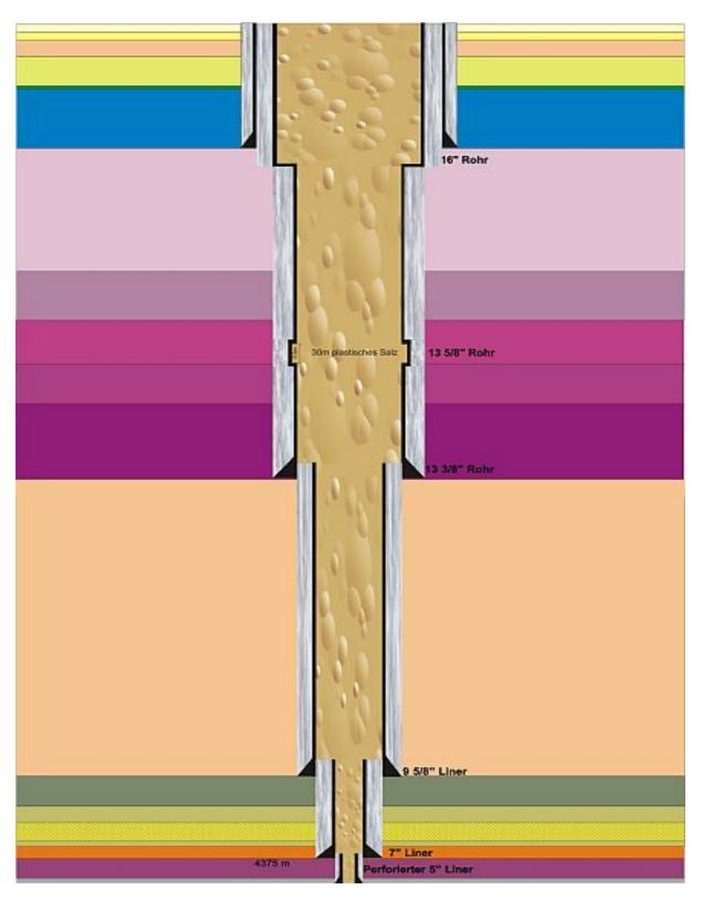
FIGURE 16: Casing completion of a borehole in deep sediments (Huenges and Moeck 2007). The grey colour indicates the cemented annulus
