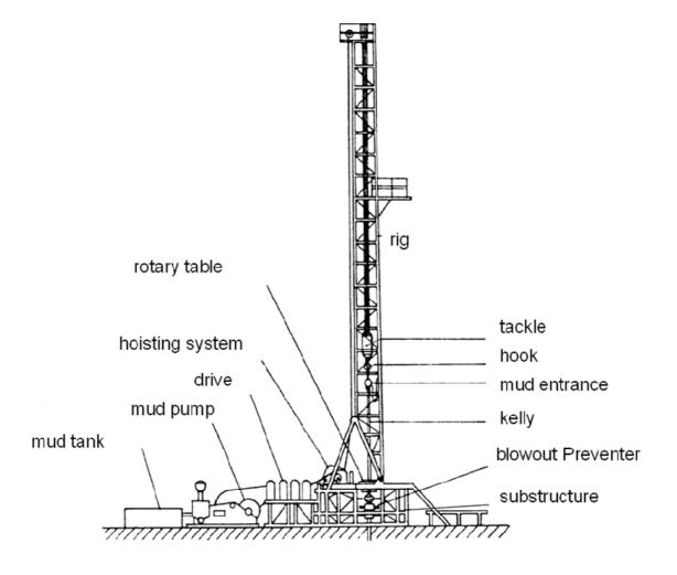
FIGURE 13: Drill rig with main components required at the drill site (Wolff 1999)
