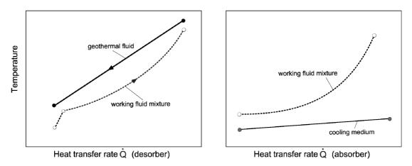
FIGURE 37: Example of a temperature-heat transfer-diagram for a Kalina cycle
