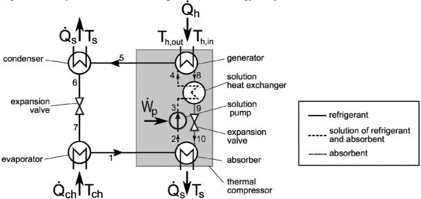
FIGURE 40: Principle of an absorption refrigeration cycle (Saadat et al., 2010)
