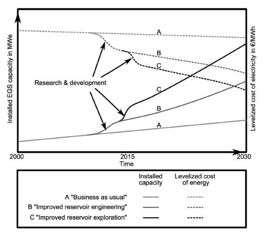
FIGURE 47: Potential development of the installed capacity and levelized cost of energy for EGS plants over time for different scenarios indicating the influence of research and development
