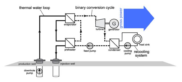
FIGURE 35: Schematic setup of an Organic Rankine cycle (ORC) (Saadat et al., 2010)
