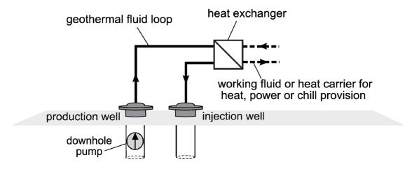
FIGURE 30: Principle for energetic use of EGS reservoirs showing a well doublet, the geothermal fluid loop and a heat exchanger on the surface (Saadat et al., 2010)
