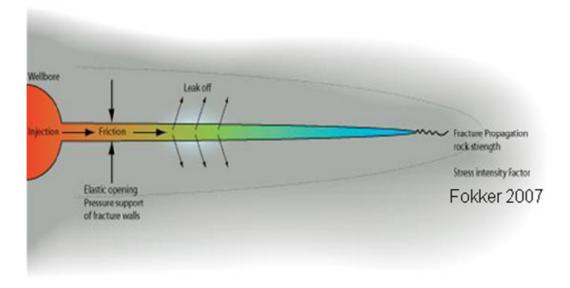
FIGURE 20: Top view of a fracture propagation due to hydraulic stimulation (Fokker, 2007)
