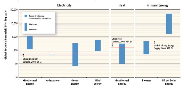
FIGURE 46: Global technical potential of renewable energy carriers which can be provided per year. The global demand of electricity and heat is given in the diagram (Edenhofer et al., 2011)
