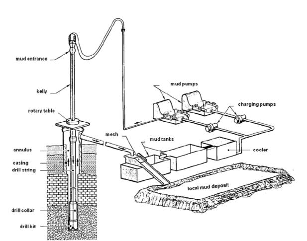
FIGURE 14: Mud circulation loop of a drilling site (Wolff, 1999)
