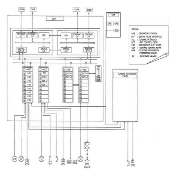
FIGURE 7: The Digital-electro-hydraulic (DEH) system at Olkaria II power plant
