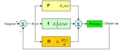
FIGURE 15: Proportional-integral-derivative (PID) controller (Wikipedia, 2008)
