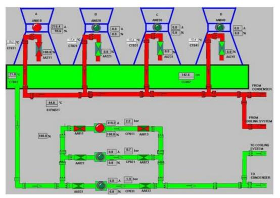
FIGURE 18: Cooling tower graphic diagram
