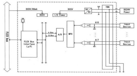
FIGURE 20: Analog input module FXAIM01 block diagram
