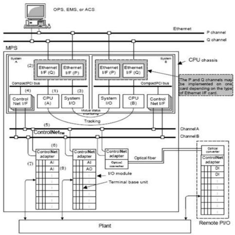
FIGURE 32: System configuration of a multiple process station
