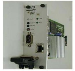
FIGURE 17: CPCPU01 Compact PCI CPU card
