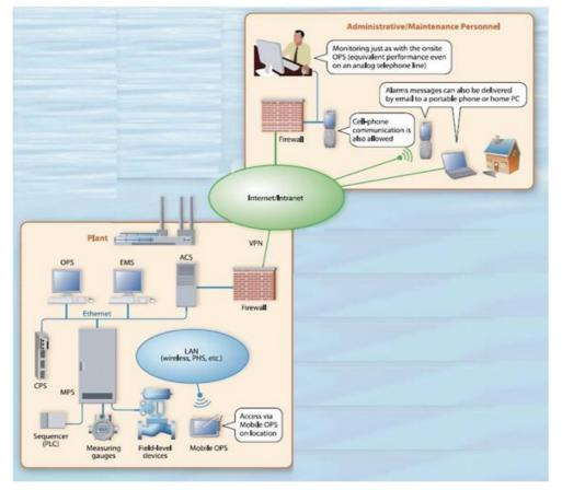
FIGURE 30: Remote monitoring and control system
