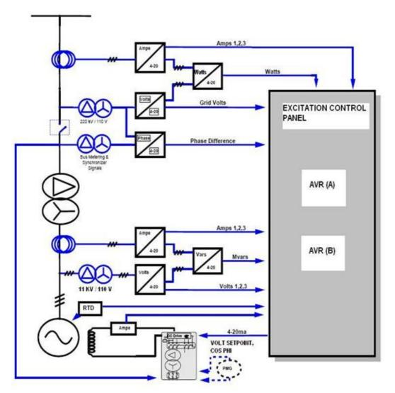
FIGURE 6: Automatic voltage regulator (AVR)
