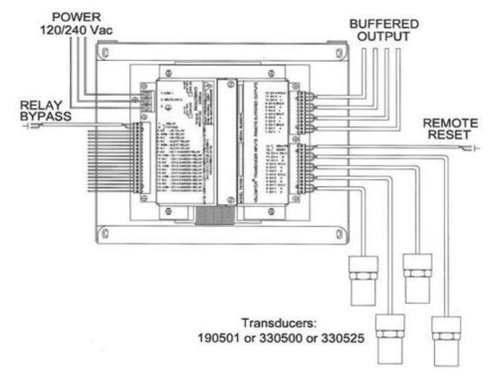
FIGURE 11: 1900/55 fan monitor and 190501 Velomitor transducers
