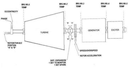
FIGURE 10: Vibration monitoring for the turbine-generator system (Rockwell, 2006)
