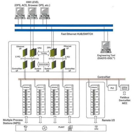
FIGURE 4: System configuration for Diasys Netmation control system at Olkaria II power plant
