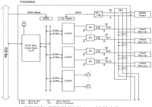
FIGURE 21: FXDIM02 digital input module block diagram
