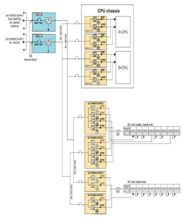
FIGURE 33: Control system power supply system (MHI, 2006b)
