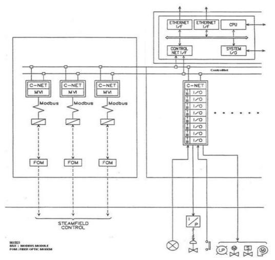
FIGURE 13: DCS interface to steamfield control
