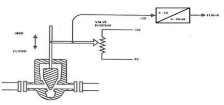
FIGURE 19: Valve position represented as an analog signal
