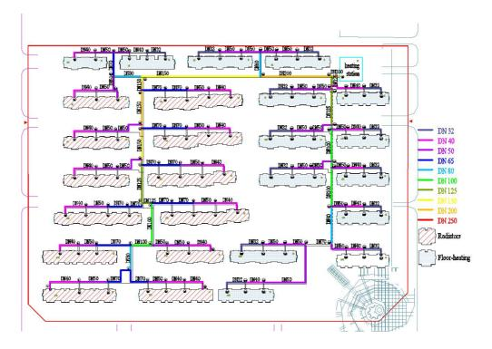
FIGURE 8: Distribution system layout for the new heating system
