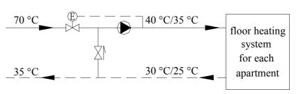
FIGURE 6: Flow chart of the new substations
