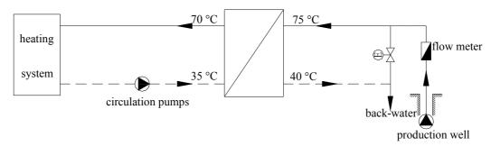
FIGURE 5: Flow chart of the new heating system
