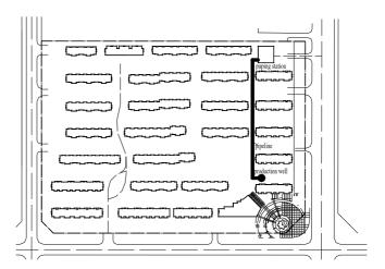
FIGURE 3: Location of geothermal well and the main hot water pipeline
