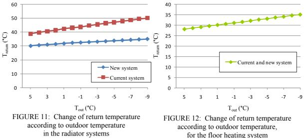
As indicated in Figure 12, in the floor heating system, the return temperature in the current system and the new system are the same. During application in winter, the highest return temperature is 35°C and the lowest is 28°C.
