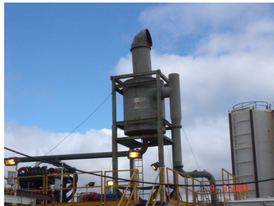
FIGURE 6: Aerated drilling separator
