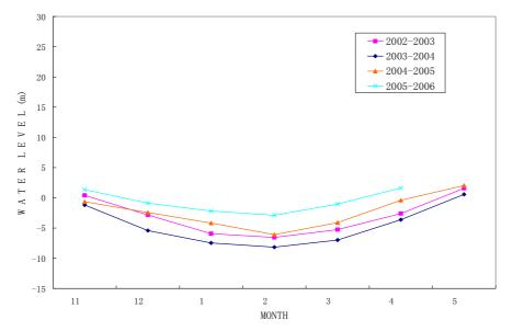
FIGURE 8: The water level of a monitoring well in Xiaotangshan geothermal field from 2002 to 2006
