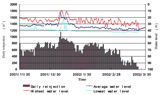
FIGURE 7: reinjection volume and water level changes of a reinjection well in the Xiaotangshan Geothermal Field during the heating season of 2001-2002
