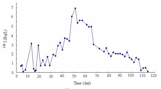
FIGURE 6: Tracer (125I) recovery of a tracer test in 2001
