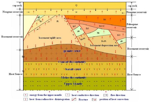
FIGURE 8: Geological geothermal model in Tianjin
