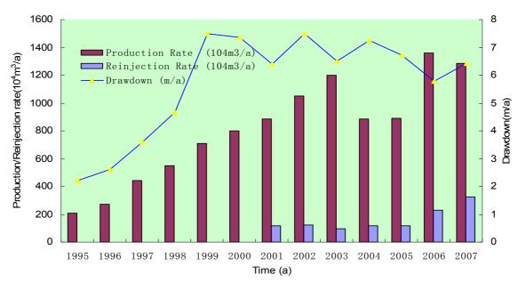
FIGURE 2: The history of water level drawdown v. geothermal water production and reinjection in the dolomite reservoir in the Tianjin urban area in 1995-2007.
