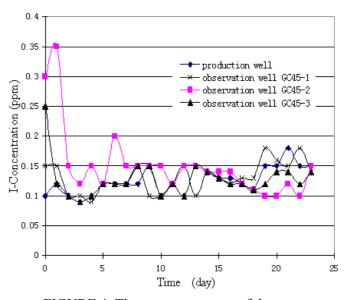
FIGURE 4: The recovery curves of the tracer concentration in the observation wells around WR45
