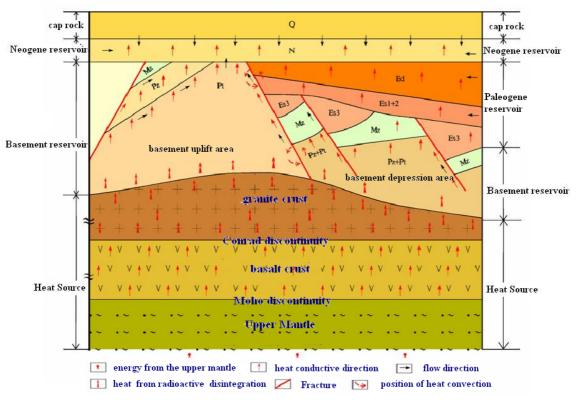
FIGURE 8: Geological geothermal model in Tianjin
