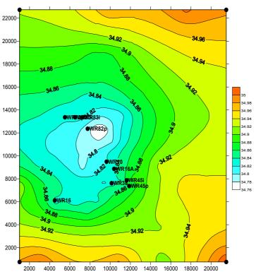
FIGURE 3: Contour map of calculated water level of the dolomite reservoir in Tianjin in Sept.2013, assuming the reinjection will increase 150%
