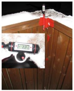
FIGURE 16: Air temperature measurement point
