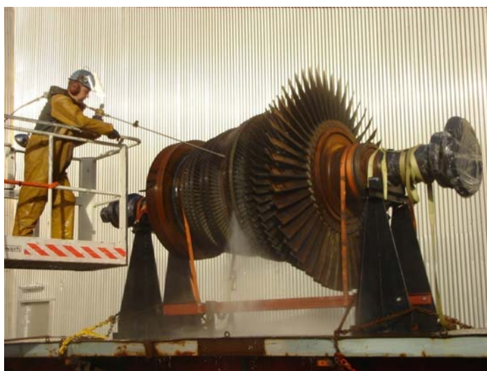
FIGURE 15: Hydro blast scale removal, Svartsengi power plant
