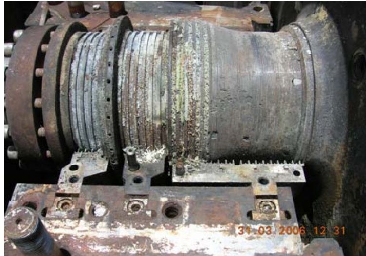
FIGURE 11: Aluto Langano GCCU labyrinth seal damage
