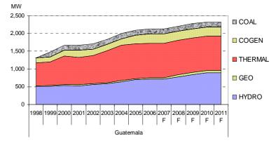
FIGURE 3: Installed capacity and projection in Guatemala (1998-2011)
