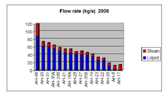
FIGURE 7: Flow rate by well
