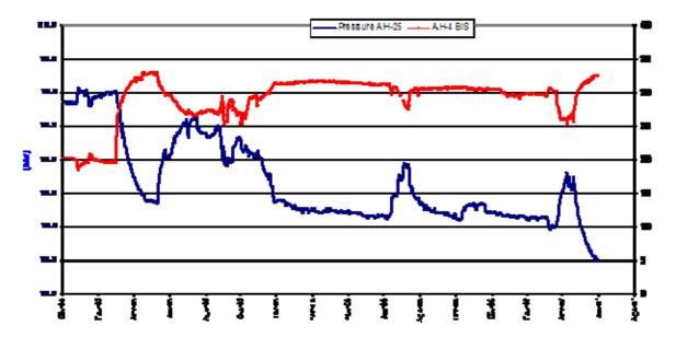
FIGURE 9: Reservoir pressure and steam flow rate in well AH-4bis
