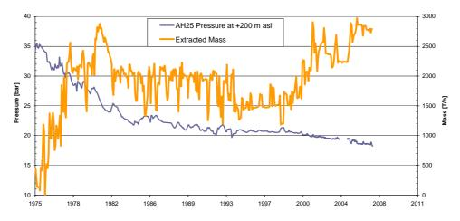
FIGURE 3: Reservoir pressure and mass extracted at Ahuachapán geothermal field
