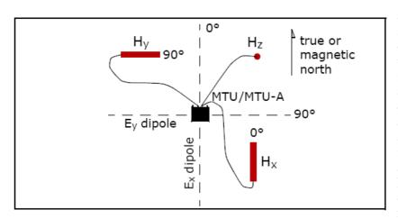
FIGURE 17: Field array for a 5-channel MT data acquisition system (Phoenix Geophysics Ltd, 2003)
