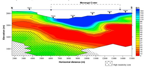
FIGURE 25: TEM resistivity cross-section NS-2
