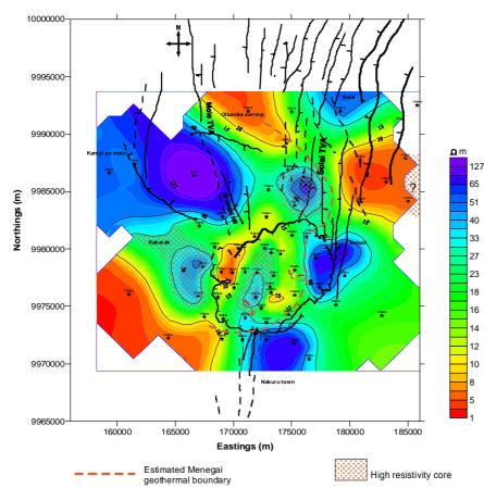
FIGURE 31: TEM resistivity distribution at 1600 m a.s.l.
