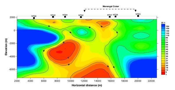
FIGURE 33: MT resistivity cross-section NW-SE
