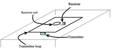
FIGURE 3: Central-loop time domain TEM layout
