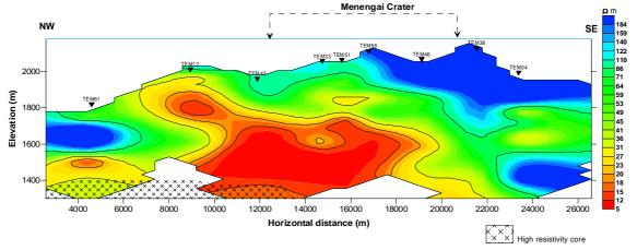
FIGURE 28: TEM resistivity cross-section NW-SE
