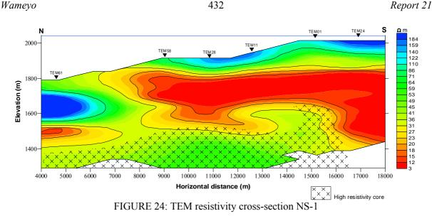
*Resistivity cross-section NS-1* is a north-south bound resistivity cross-section, passing west of the caldera (Figure 24). It shows a low-resistivity layer sloping down to the north. It is underlain by higher resistivity except in the far south.
