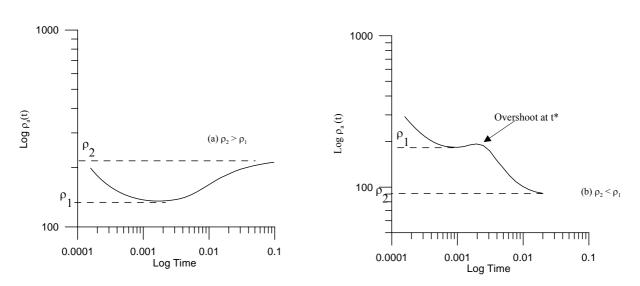
FIGURE 10: TDEM - apparent resistivity, two layered earth, a)  $\rho_2 > \rho_1$ ; b)  $\rho_2 < \rho_1$
