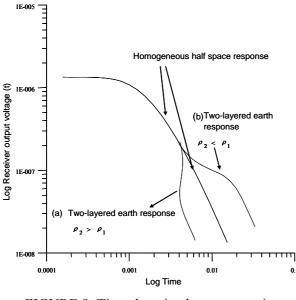
FIGURE 9: Time domain electromagnetic (TDEM) receiver output voltage, two layered earth
