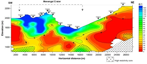
FIGURE 29: TEM resistivity cross-section NE-SW
