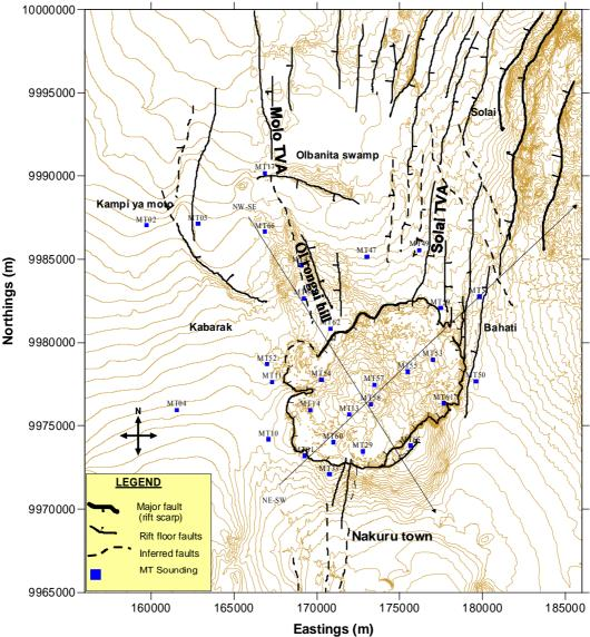
FIGURE 16: Map showing location of MT soundings and resistivity cross-sections
