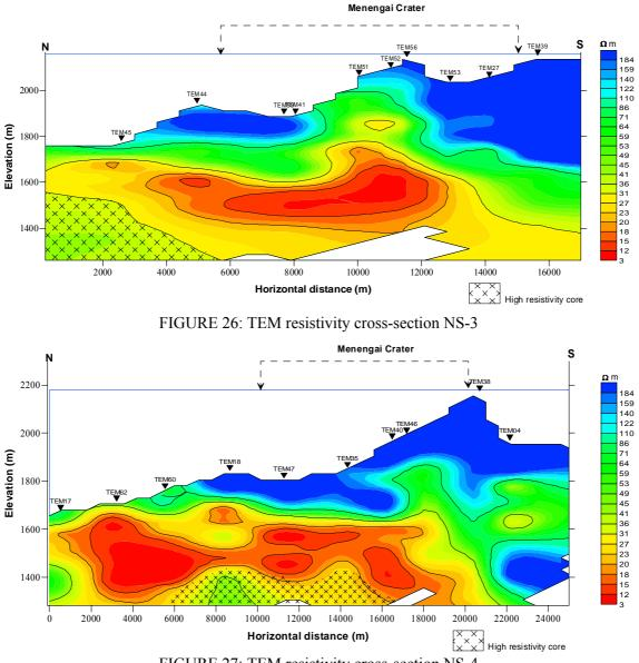
FIGURE 27: TEM resistivity cross-section NS-4
