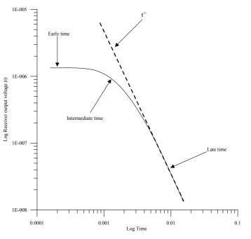
FIGURE 7: Log plot of receiver output voltage versus time
