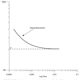
FIGURE 8: Apparent resistivity of a half-space versus time
