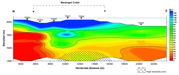
FIGURE 22: TEM resistivity cross-section EW-6
