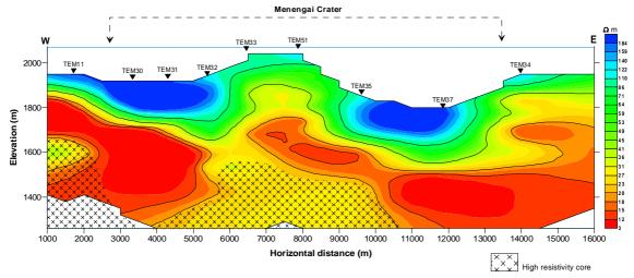
FIGURE 20: TEM resistivity cross-section EW-4
