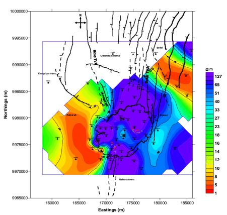
FIGURE 30: TEM resistivity distribution at 1800 m a.s.l.
