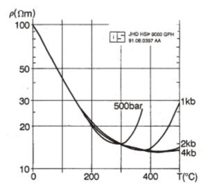
FIGURE 2: Resistivity of an electrolyte as a function of temperature at different pressures (mod. from Quist and Marshall, 1968)
