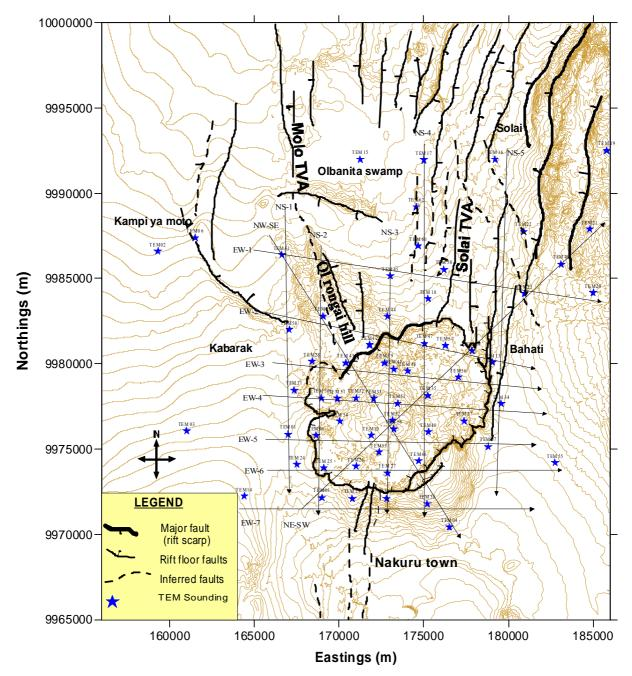
FIGURE 15: Map showing location of TEM soundings and resistivity cross-sections
