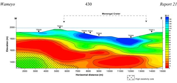
FIGURE 19: TEM resistivity cross-section EW-3
