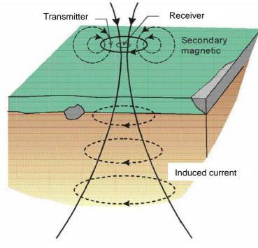
FIGURE 6: Transient current flow in the ground (mod. from Hersir and Björnsson, 1991)
