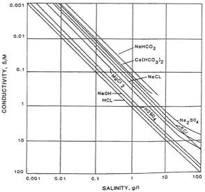
FIGURE 1: Pore fluid conductivity vs. salinity (concentration) for a variety of electrolytes (modif. from Keller and Frischknecht, 1966)
