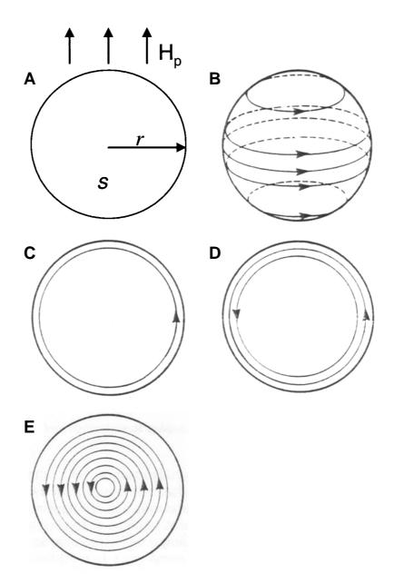
FIGURE 5: Target conductive sphere and current distribution
