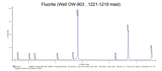
FIGURE 15: Diffractogram of fluorite showing a strong peak at 3.156 Å
