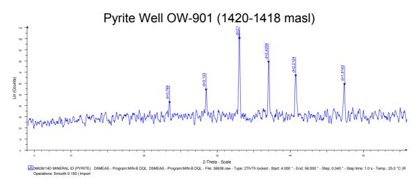
FIGURE 18: Diffractogram of pyrite showing strong peaks at 3.13 Å, 2.71 Å, 2.42 Å, 2.21 Å and 1.91 Å
