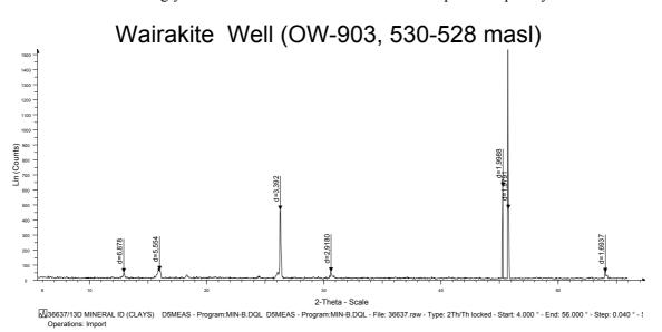
FIGURE 21: Diffractogram of wairakite showing strong peaks at 3.92 Å and at approximately 2.00 Å
