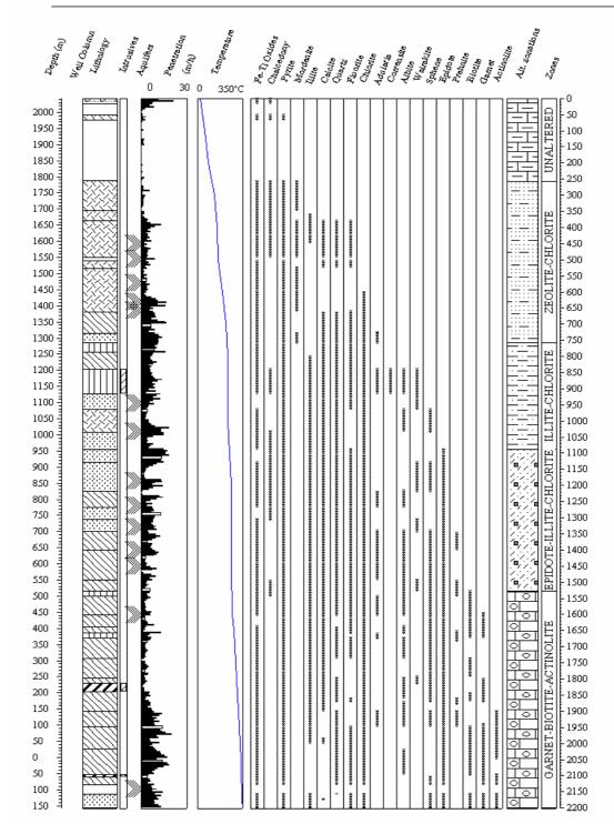
FIGURE 12: Lithology, distribution of hydrothermal alteration minerals and zonations in well OW-903. Legend on lithology is as in Figure 9
