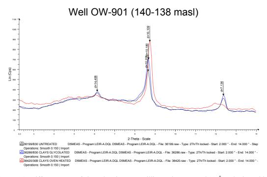
FIGURE 16: Diffractograms of clays showing strong illite peaks at around 10 Å and minor chlorite component with peaks at 7.14 Å and at 14.41 Å in the untreated, glycolated and the oven heated runs
