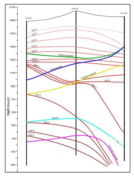
FIGURE 27: Plot of epidote, illite, chlorite, actinolite and garnet isograds and measured temperature isotherms across wells OW-901, OW-903 and OW-902
