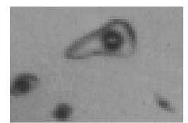
PLATE 2: Fluid inclusion in hydrothermal calcite with a homogenization temperature of 320°C at 240 masl in well OW-901
