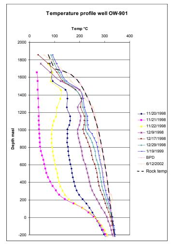
FIGURE 28: Temperature profiles of well OW-901
