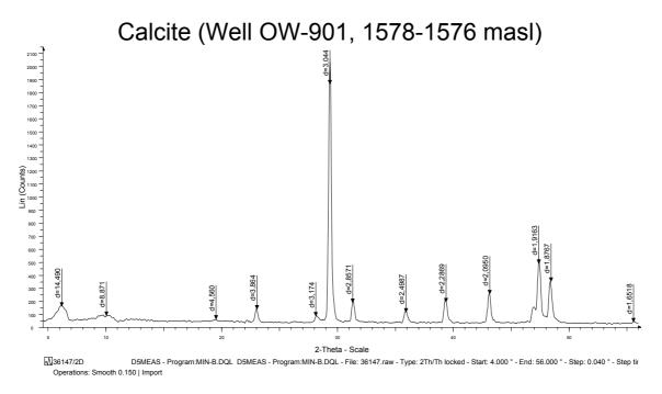
FIGURE 13: Diffractogram of calcite showing a strong peak at 3.044 Å
