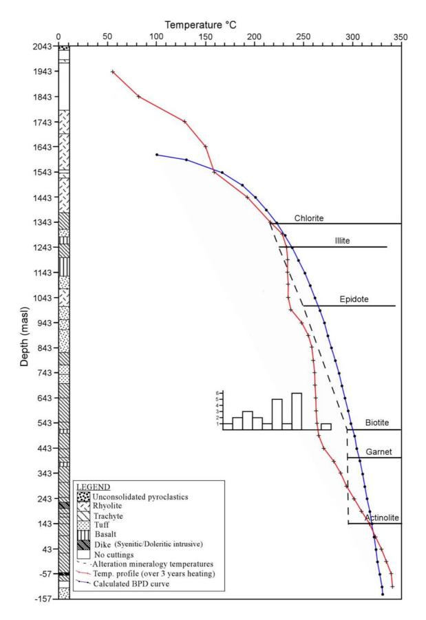
FIGURE 26: Plot of lithology and correlation between measured, interpreted hydrothermal alteration minerals and fluid inclusion temperatures with depth of well OW-903
