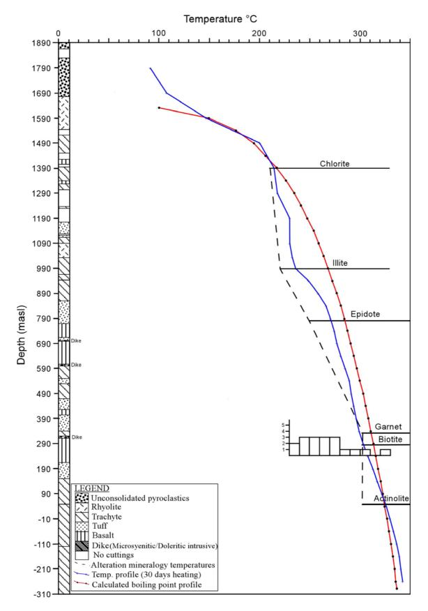
FIGURE 24: Plot of lithology and correlation between measured, interpreted hydrothermal alteration minerals and fluid inclusion temperatures with depth of well OW-901
