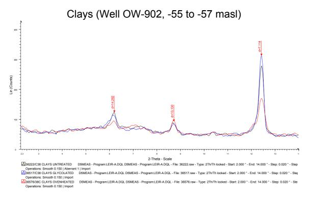
FIGURE 14: Diffractograms of clays showing unchanged peaks at 7.11 Å and 14.26 Å for chlorite and 10.13 Å for illite in the untreated, glycolated and the oven heated runs
