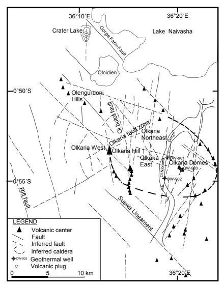
FIGURE 4: Structural map of Greater Olkaria geothermal area based on SPOT satellite image and aerial photographs. Modified from Muchemi (1992) and Mungania (1992)
