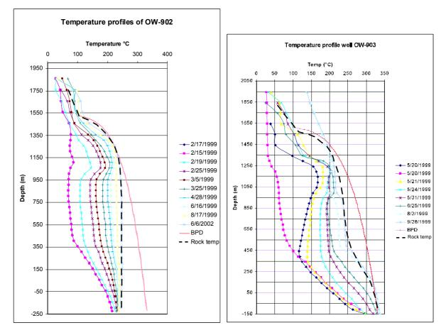
FIGURE 29: Temperature profiles of well OW-902
