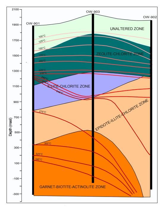
FIGURE 22: Distribution of zonations and measured formation temperature isotherms with depth across wells OW-901, OW-903 and OW-902 in Olkaria Dome field
