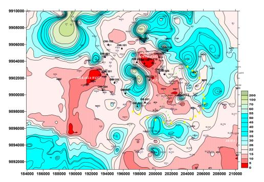
FIGURE 5: Integrated TEM and DC Schlumberger resistivity ( $\Omega$ m) at 1000 masl (KenGen, 2000). The gray/yellow stars represent the ring fracture
