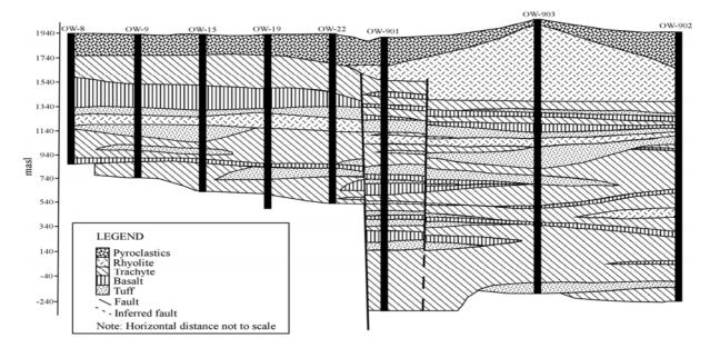
FIGURE 9: Geological cross-section along A-B-C-D (see Figure 3) between Olkaria East and Olkaria Domes fields. Correlation through wells OW-8, OW-9, OW-19 and OW-901 modified from Omenda (1999)
