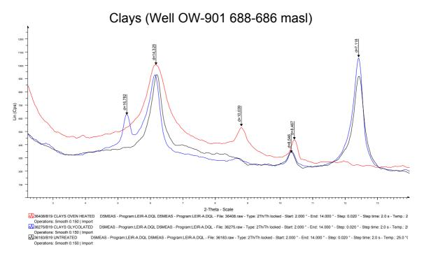
FIGURE 19: Diffractograms of clays showing swelling chlorite peaks at 14.28 Å for the untreated run, the glycolated run swells to 16.78 Å and the oven heated run collapses to 14.33 Å. Illite and chlorite are also present in the analysed sample
