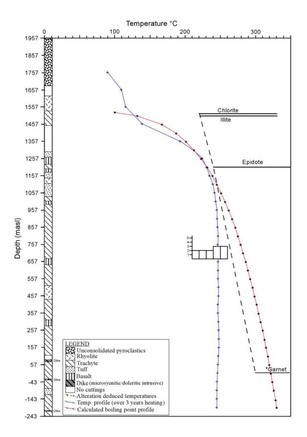
FIGURE 25: Plot of lithology and correlation between measured, interpreted hydrothermal alteration minerals and fluid inclusion temperatures with depth of well OW-902. \*Based on electron microprobe analysis Karingithi (2002)
