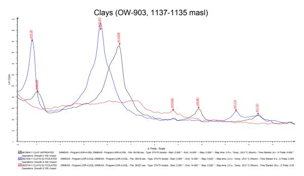
FIGURE 20: Diffractograms of clays showing strong corrensite 001 peak at 29.10 Å for the untreated run, the glycolated run swell to 31.60 Å and the oven heated run collapses completely, the 002 peaks are at 13.56 Å and 15.47 Å for the untreated and the glycolated runs while the oven heated collapses completely
