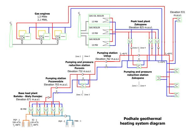
FIGURE 4.8: Technical diagram of the geothermal heating system under construction in the Podhale region (Dlugosz, 2003)
