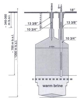
FIGURE 2.10: A sketch of a chamber formed as a result of salt brine underground leaching method and used for underground storage (based on Bujakowski [ed.] et al., 2003)
