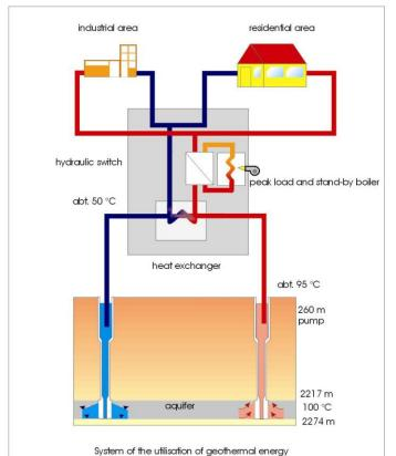
FIGURE 2.3: A scheme of the Neustadt-Glewe geothermal space-heating plant, Germany (Menzel et al., 2000)
