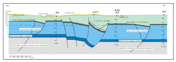
FIGURE 3.6: Geological cross-section through Slomniki area, S-Poland
