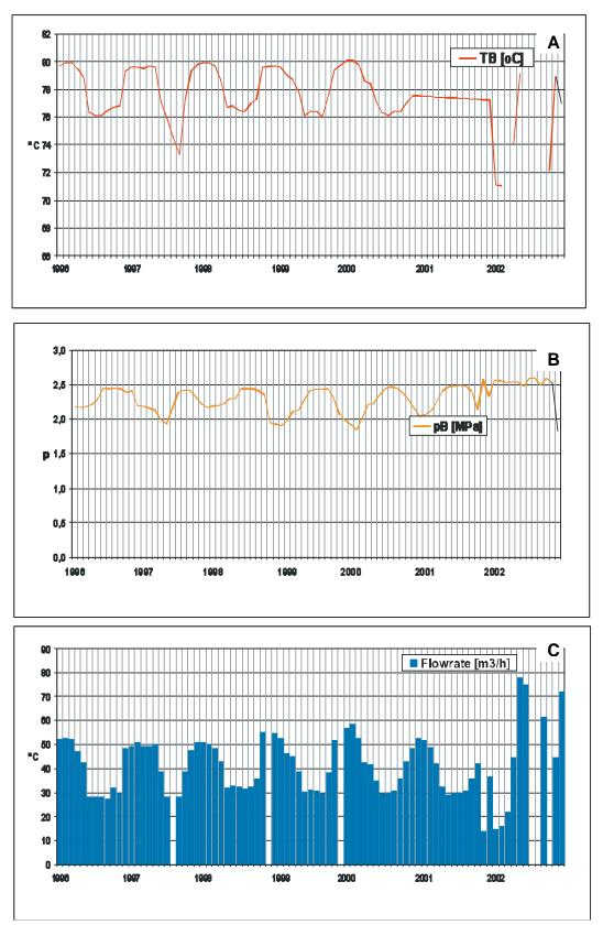
FIGURE 4.15: The Podhale geothermal system– production history of Banska IG-1– Bialy Dunajec PAN-1 doublet of wells, 1995-2001 A. Temperature; B. Pressure; and C. Flow rate (period of stable surface installations' conditions; in late 2001 the exploitation was expanded by new production and injection wells)
