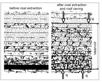
FIGURE 2.6: Sketch of water reservoir in the mine workings after extraction of coal seam (black layer) and caving in of the roof; arrows q mark heat inflow (Malolepszy, 2003)
