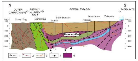
FIGURE 4.3: Geological – thermal cross-section through the Podhale region (geology based on Sokolowski, 1993, updated)
