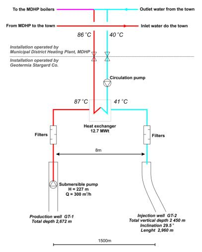
FIGURE 3.8: Stargard Szczecinski - a sketch diagram of a geothermal plant (Kozlowski and Malenta, 2002)
