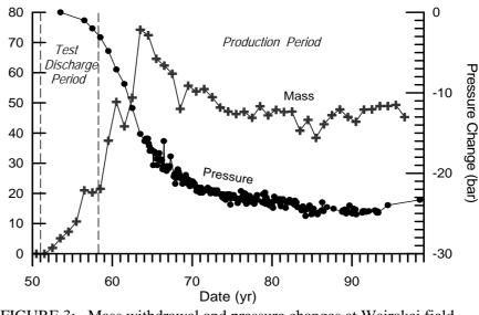
FIGURE 3: Mass withdrawal and pressure changes at Wairakei field, pressure is on average at -152 m a.s.l.; taken from Hunt & Glover (1996) and updated
