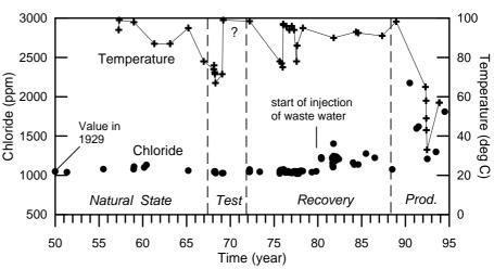
FIGURE 18. Changes in temperature and chloride concentration in Ohaaki Pool; note the lack of change in chloride concentration until after injection of waste water began. Taken from Glover et al. (2000)
