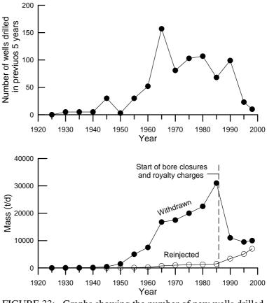
FIGURE 33: Graphs showing the number of new wells drilled and mass of fluid withdrawn and reinjected at Rotorua City; note the decrease in number of new wells drilled and increase in the amount of fluid reinjected following imposition of economic measures
