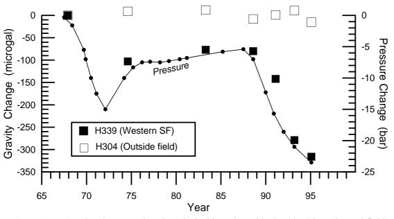
FIGURE 37: Gravity changes at benchmarks inside and outside the Ohaaki geothermal field. Note how the gravity changes at benchmark H339 (near centre of Western steamfield) follow the reservoir pressure changes
