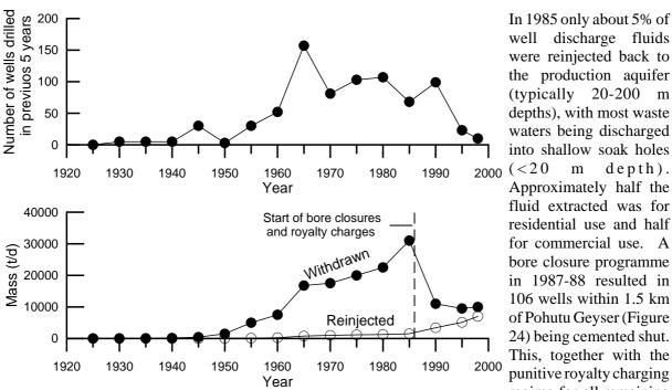
FIGURE 25: History of wells drilled in Rotorua, and the amounts of fluid withdrawn and reinjected; note the rapid decrease in mass withdrawn and increase in mass reinjected following the start of bore closures and imposition of royalty charges. Data from Scott & Cody (2000)
