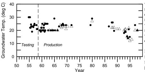
reliable and more variable than level measurements because of difficulties inherent in measuring temperature, water level changes and steam heating effects, as well as short-term climatic effects.
