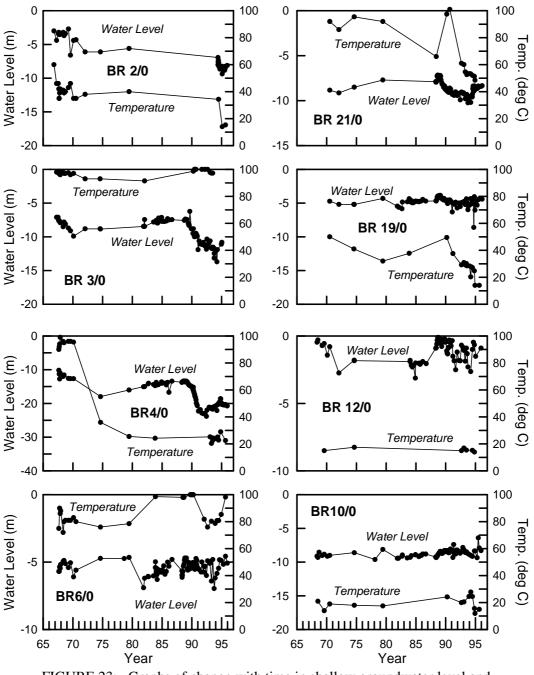
FIGURE 23: Graphs of change with time in shallow groundwater level and groundwater temperature at Ohaaki field; taken from Hunt & Bromley (2000)
