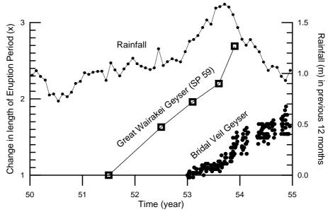
FIGURE 7: Changes in length of eruption period  $(T/T_0)$  of geysers in Geyser Valley at Wairakei during the test discharge period; periods are normalised to  $T_0 = 12.5$  hours for Great Wairakei Geyser, and 39 min for Bridal Veil. Rainfall data are monthly running totals of rainfall in previous 12 months. Note the steady increase in length of eruption period with time
