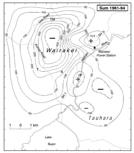
FIGURE 35: Sum of measured gravity changes from 1961 (first survey) to 1994 (last field- wide survey) at Wairakei geothermal field, New Zealand. Contour values at 50 microgal intervals; zero contour has been omitted for clarity. Map has been constructed by summation of 500 m grid values obtained from the maps in previous figure
