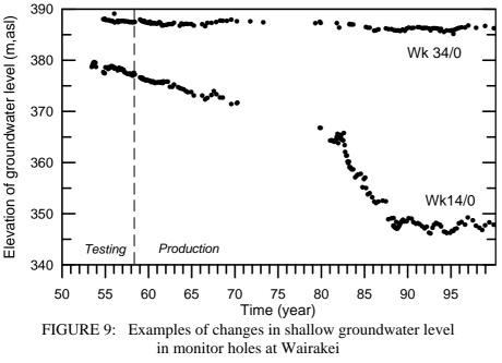
Groundwater levels have been monitored in shallow (20-50 m depth) holes since 1953. In most places the water level has varied by about  $\pm 1$  m in response to seasonal variations in rainfall (for example 34/0.Figure 9). However, in monitor holes in an area adjacent to the Western borefield the levels have fallen significantly. These holes are situated near a region of cold water invasion, and it is believed that a large part of the cold downflow
