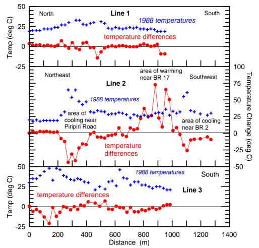
FIGURE 22: Changes in shallow ground temperatures at Ohaaki field, temperature differences are for the period 1988-1996, and cover the first 8 years of the production period. The differences have been adjusted for seasonal differences; location of the survey lines are shown in Figure 19. Taken from Hunt & Bromley (2000)
