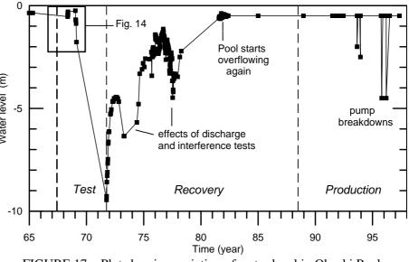
FIGURE 17: Plot showing variation of water level in Ohaaki Pool with time; note the rapid recovery of water level after end of the test discharge period. Taken from Glover et al. (2000)
