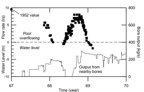
FIGURE 16: Plot showing variation of flow rate and water level in Ohaaki Pool during the early part of the test discharge period at Ohaaki field; note the rapid response of flow rate to changes in output from nearby bores being test discharged. Taken from Glover et al. (2000)
