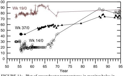
FIGURE 11: Plot of groundwater temperatures in monitor holes in part of the production area at Wairakei; note the increase in temperature in some holes
