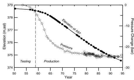
FIGURE 14: Change in elevation (subsidence) of benchmark A97 compared with deep liquid pressure changes at Wairakei, note that the subsidence has continued despite stabilisation of pressure since late 1970's. Data from Hunt & Glover (1996)
