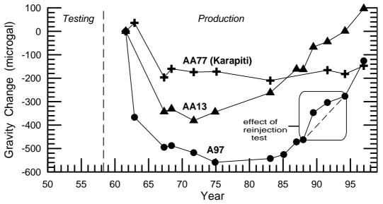
FIGURE 36: Gravity changes at selected benchmarks in Wairakei geothermal field, New Zealand. Benchmarks AA13 and A97 are in the Eastern borefield. Note the gravity decreases during the early stages of production as the 2-phase zone expanded, followed by the gravity increases as the deep water level in the Eastern borefield rose as the rocks became re-saturated as a result of cold downflows
