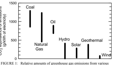
FIGURE 1: Relative amounts of greenhouse gas emissions from various types of electricity generation methods, data expressed as  $CO_2$  equivalents; taken from Geothermal Energy News (May 1998), and geothermal data adjusted on basis of data from ETSU (1998)
