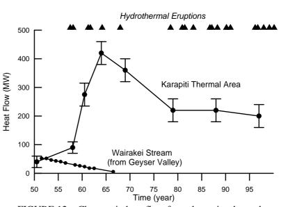
FIGURE 12: Changes in heat flow from the major thermal areas of Wairakei field; taken from Hunt et al. (1998)
