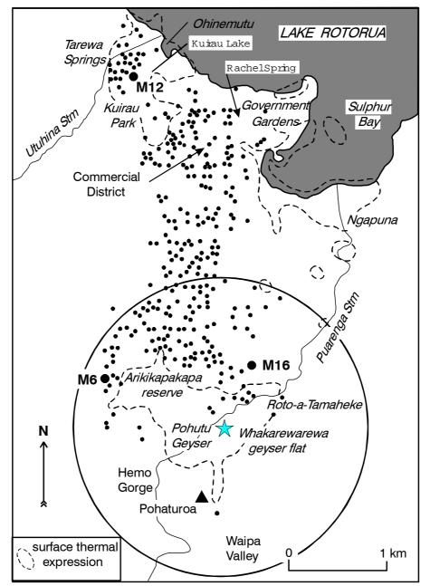
FIGURE 24: Distribution of geothermal wells in Rotorua City in 1985 (solid dots), monitor wells and thermal areas (outlined by broken lines); circle shows area in which all geothermal wells were closed. Taken from Scott & Cody (2000)
