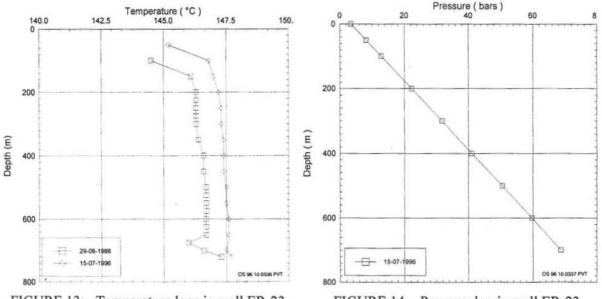
FIGURE 13: Temperature logs in well ER-23
