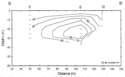
FIGURE 6: Temperature cross-section B-B', across the Efri-Reykir anomaly from south to north
