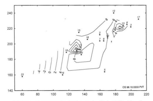
FIGURE 9: Contour map showing the water level in the Efri-Reykir wells
