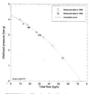
FIGURE 11: The plot of wellhead pressure vs. total flow
