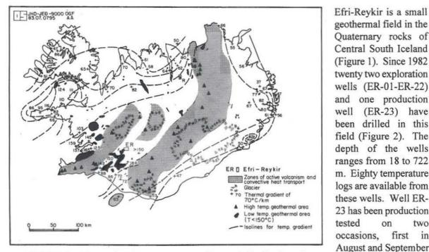
Quaternary rocks of Central South Iceland (Figure 1). Since 1982 twenty two exploration wells (ER-01-ER-22) and one production well (ER-23) have been drilled in this field (Figure 2). The depth of the wells ranges from 18 to 722 m. Eighty temperature logs are available from these wells. Well ER-23 has been production tested on two occasions, first in August and September 1988 (Jónsson et al., 1988) and later in July 1996 (Björnsson and Steingrímsson, 1996).
