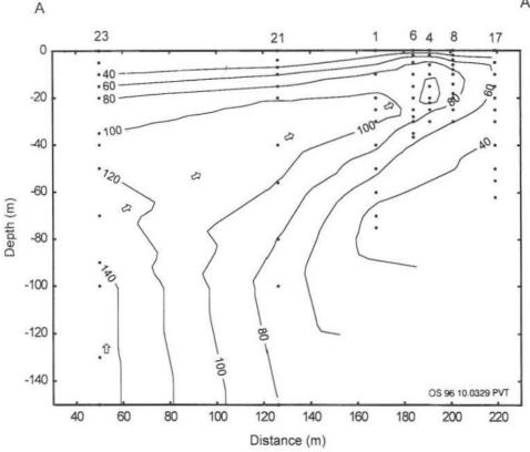
FIGURE 5: Temperature cross-section A-A', along the Efri-Reykir anomaly
