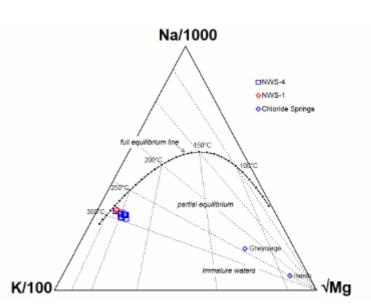
FIGURE 8: Giggenbach's geoindicator ternary diagram
