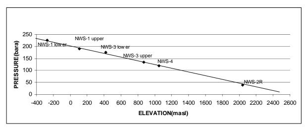
FIGURE 6: Pressure profile with depth (PCP plot)
