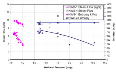
Well NWS-1 was successfully discharged on 28th May 2004 until being shut on 18th June 2004, for a period of 21 days. The well initially flowed at a WHP of about 3.3 bar-g until the flow stabilised and was then throttled until the WHP reached 4.1 bar-g. Prior to shutting NWS-1 was on discharge to the silencer and the WHP reached a maximum value of 4.5 bar-g. After the initial discharge period there was little change in discharge enthalpy, which stabilised at close to 1000 kJ/kg (Figure 7)
