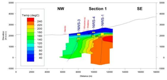
FIGURE 5: Sabalan vertical-section temperature contours
