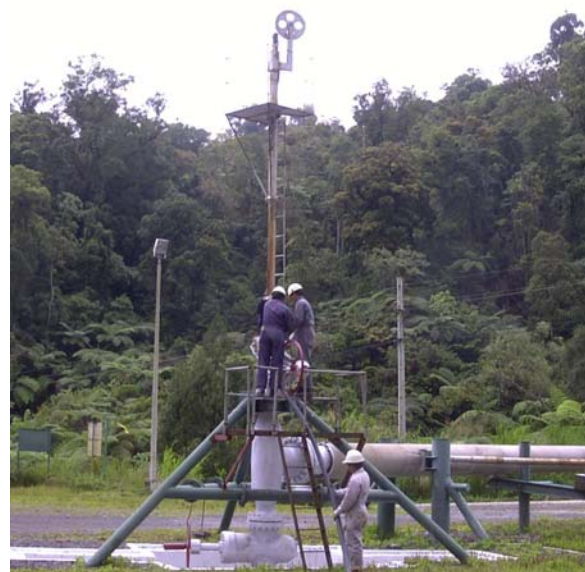
FIGURE 3: CIS set-up in well APO-1D (MGPF)
