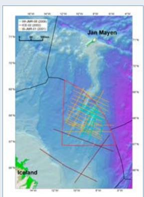
3600 km of seismic reflection lines acquired in 2001 and 2008 by CGGVeritas. 800 km aquired by TGS-NOPEC in 2002.
