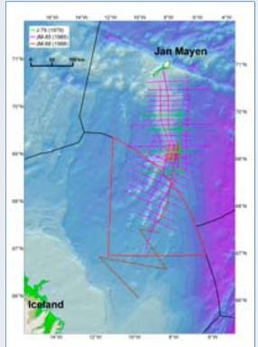
Approximately 5800 km of seismic reflection lines acquired by Norway in 1979, and by Iceland and Norway in 1985 and 1988. Reprocessed data of 1985 and 1988 surveys available from Spectrum.
