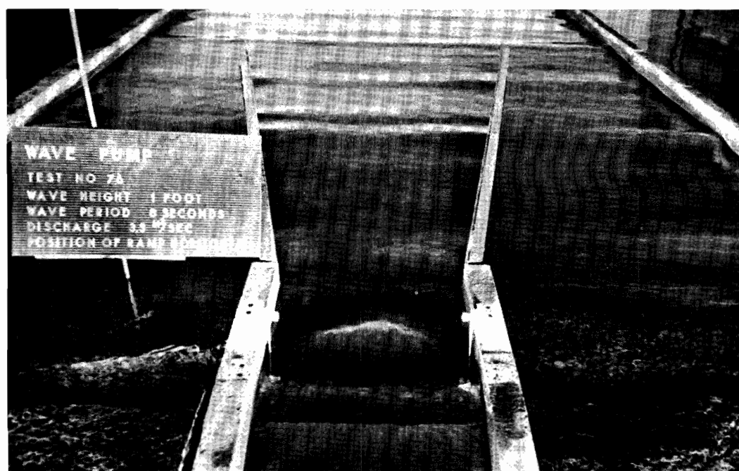
Photo 4 Test no 76, wave height 1 ft, wave period 8 sec, discharge 3,3 m 3 /sec, position of ramp horizontal
