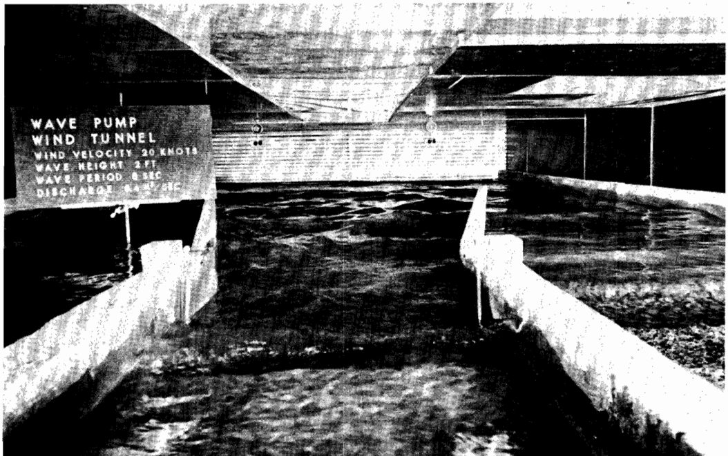
Photo 12 Wind tunnel, wind velocity 20 knots, wave height 2 ft, wave period 8 sec, discharge 8,4 \text{ m}^3/\text{sec} .
