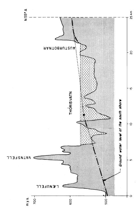
Fig. 6. Longitudinal section of Lake Thórisvatn showing the piezometric surface along its SE shore.
